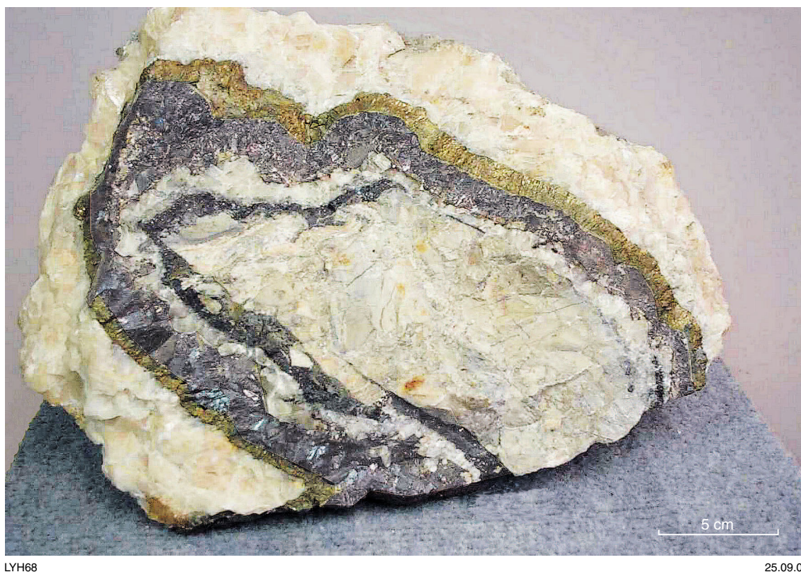
Figure 23. Photograph of Goongewa ore: sphalerite and galena with marcasite and sparry calcite surrounding a limestone fragment in a solution cavity
