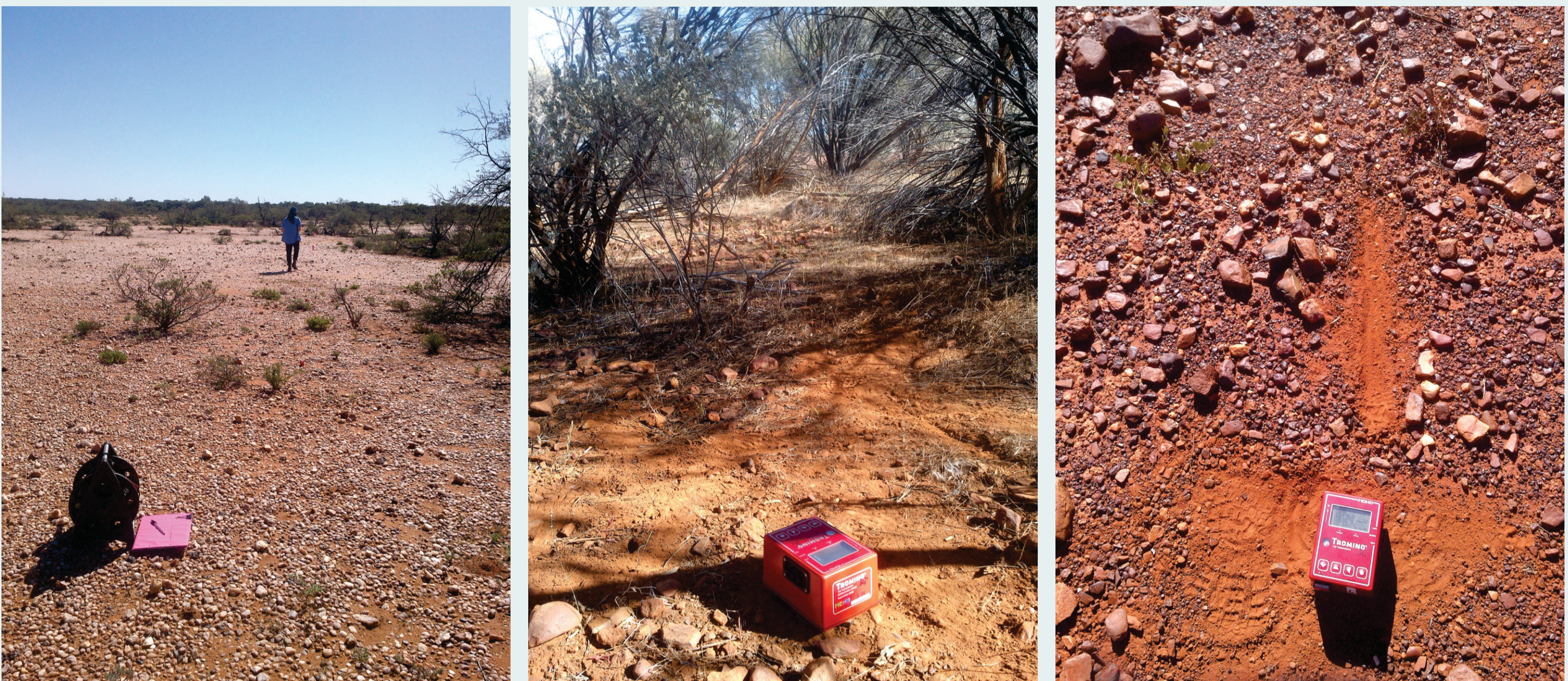
Figure 2. Field photos showing the typical sandy, lag dominated cover of the project area and two shallow passive seismic sites with Tromino instruments
