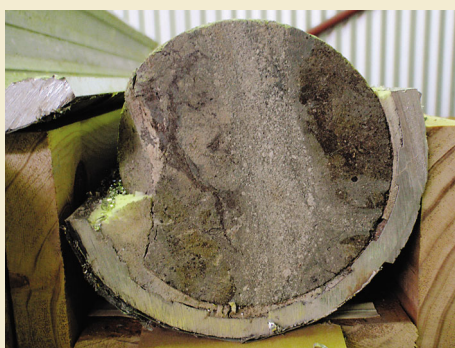
End-core photographs of core from the basal section of the upper Lesueur Sandstone showing sedimentary features
