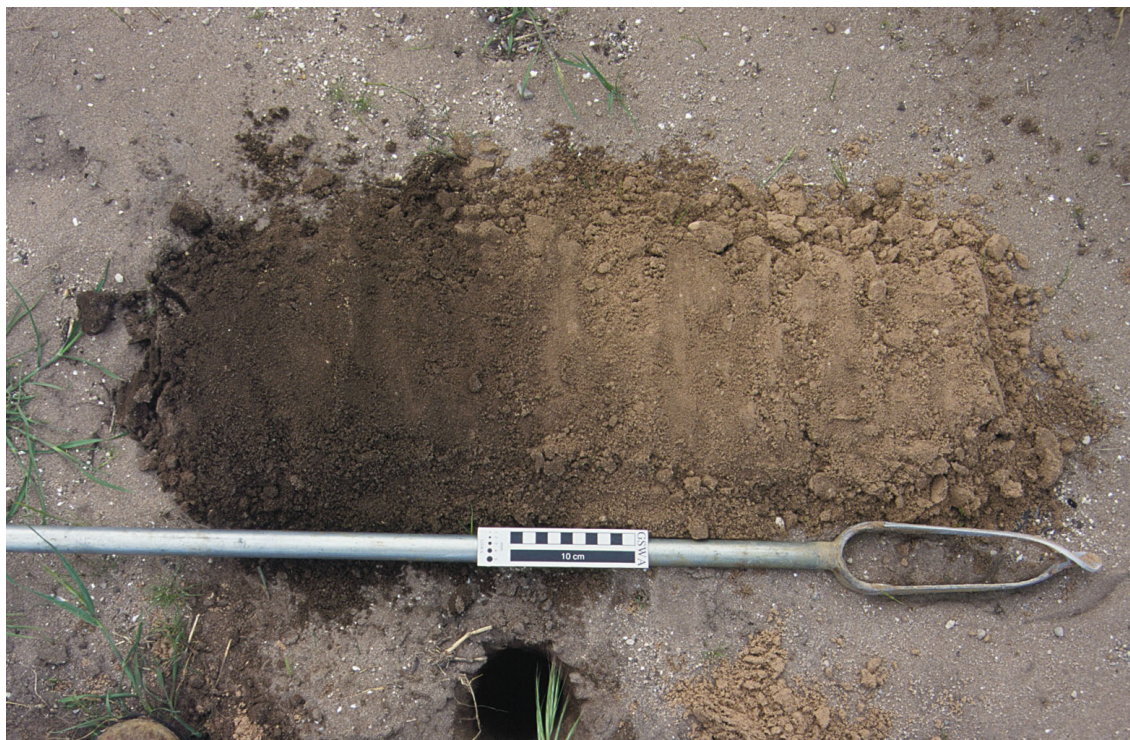
Figure 35. Soil auger sample from older, deflated dunes ( QuE2 ) 3 km north of Oakajee, composed of light brown 7.5YR 6/4 calcareous soil with moderately weak calcarenite nodules (MGA 262470E 6838725N; GSWA Photograph No. 1357)
