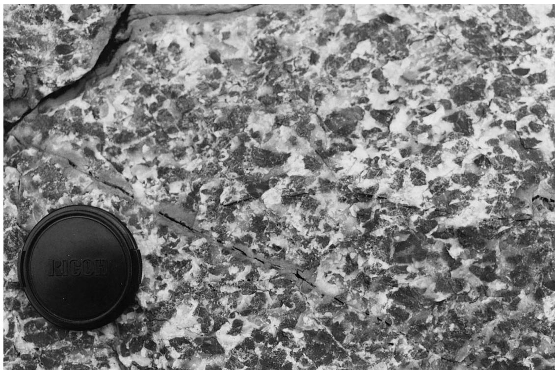
Figure 5. Chert breccia (?hydrothermal) along a faulted contact between the Johnson Cairn and Doolgunna Formations (AMG 953188). The lens cap is 5.5 cm in diameter
