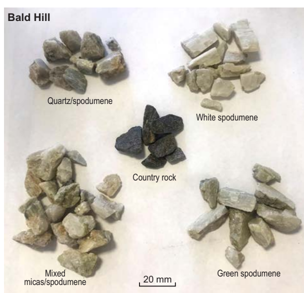
Figure 106. Examples of concentrates showing spodumene with variation in colour and the presence of gangue minerals, which have been collected along with spodumene in the beneficiation circuits
