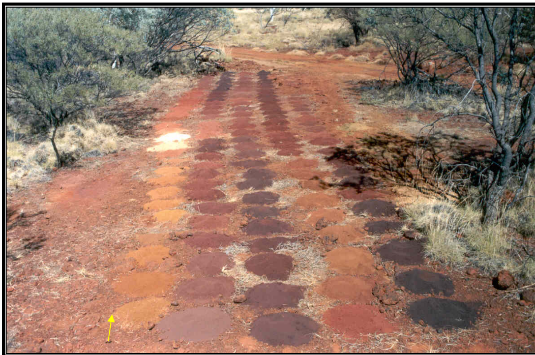
Photo 69. 1 m RC drill samples showing a large range in colour corresponding to conglomeratic (darker reds to purples) to more silty and shaly facies (pinks to browns), top of hole arrowed, GLR0006, L Deposit, Southern Flank.
