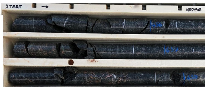
Figure 5: Dominant basement rock groups identified downhole in NDD1901.
