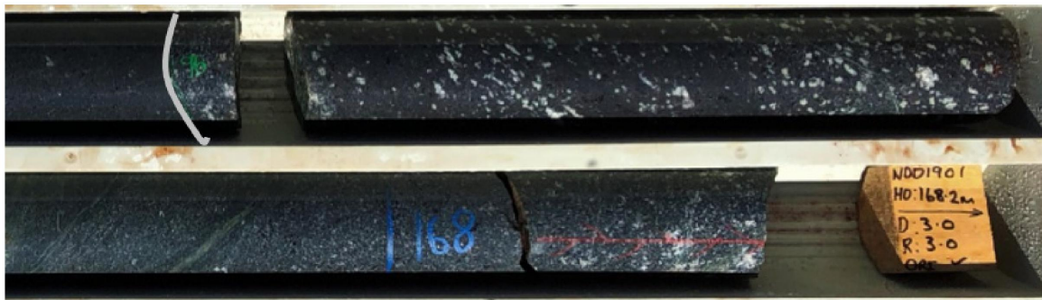
Figure 7: Mafic-intermediate porphyry in NDD1901.
