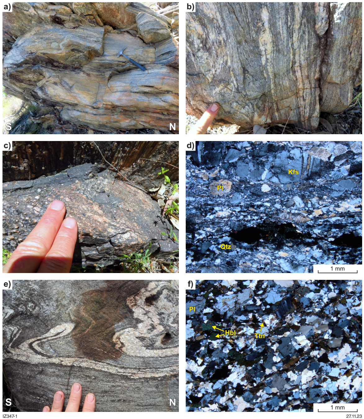
Figure 3. Outcrop-scale and microscale features of the main layered rock types identified within the CMB: a) layered granitic migmatite gneiss, showing its typical centimetre-to-decimetres-scale compositional layering, with alternating melanocratic (biotite-rich) and leucocratic layers; b) close-up view from the same outcrop shown in a), highlighting the competency contrast between the stronger leucocratic layers (which are boudinaged) and the weaker, biotite-rich layers; c) close-up view of a melanocratic layer, which contains up to 90% biotite, probably representing a restitic layer resulting from migmatization; d) typical microstructure of layered migmatite gneiss shown in a), with plagioclase (Pl) and K-feldspar (Kfs) porphyroclasts wrapped by quartz ribbons (Qtz). Crossed polars in all micrographs presented here, unless indicated; e) typical appearance of the amphibole-bearing tonalitic migmatite gneiss, with layering defining refolded folds; f) typical microstructure of layered migmatite gneiss shown in e), with hornblende (Hbl) and titanite (Ttn) aggregates surrounded by plagioclase (Pl) and quartz porphyroclasts.
