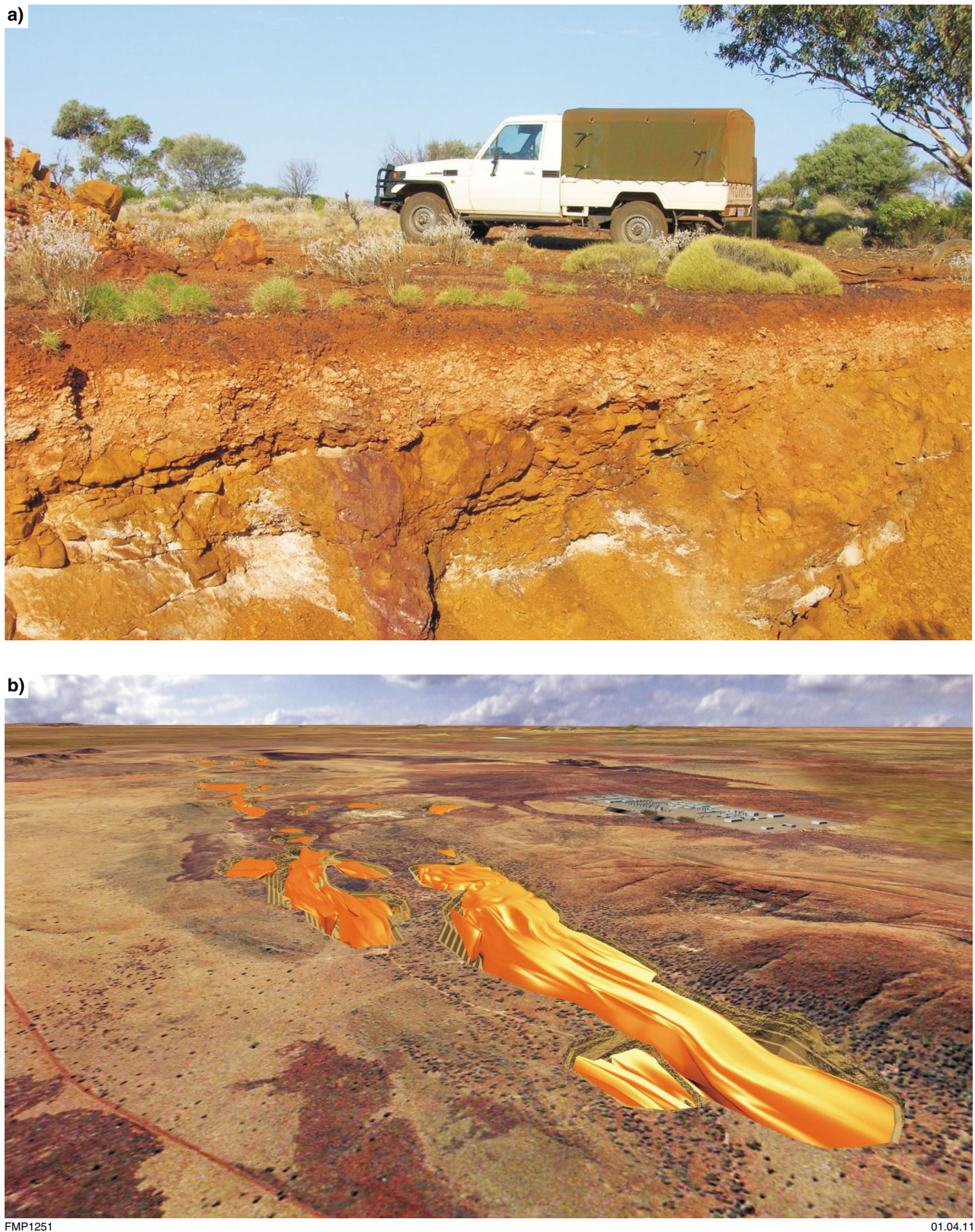
Figure 46. a) Wingellina nickeliferous ochre material, exposed in an exploration costean; b) 3D computer model of nickel orebody (from Metals X Ltd, < http://metalsx.com.au/operations/wingellina_nickel/ >)
