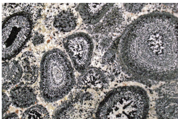
Figure 5. A polished tile of Boogardie orbicular granite. The hornblende diorite orbicules are composed largely of white plagioclase feldspar, and large, black, radially aligned hornblende crystals.
