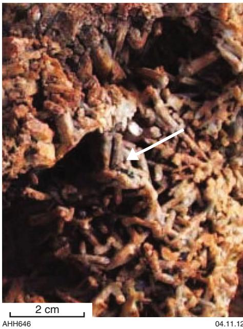
**Figure 19. Euhedral hydrothermal quartz filling an open cavity**
