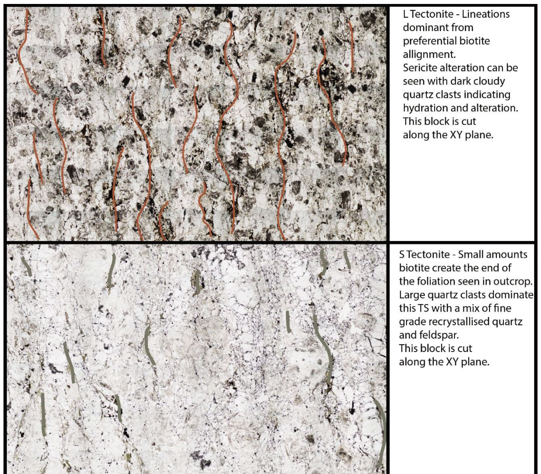
Figure 17e – L Tectonite vs S tectonite thin section images. Lineations extend throughout the L tectonite via biotite stretching. The biotite in the S tectonite can be seen to be cut off while creating the foliation.
