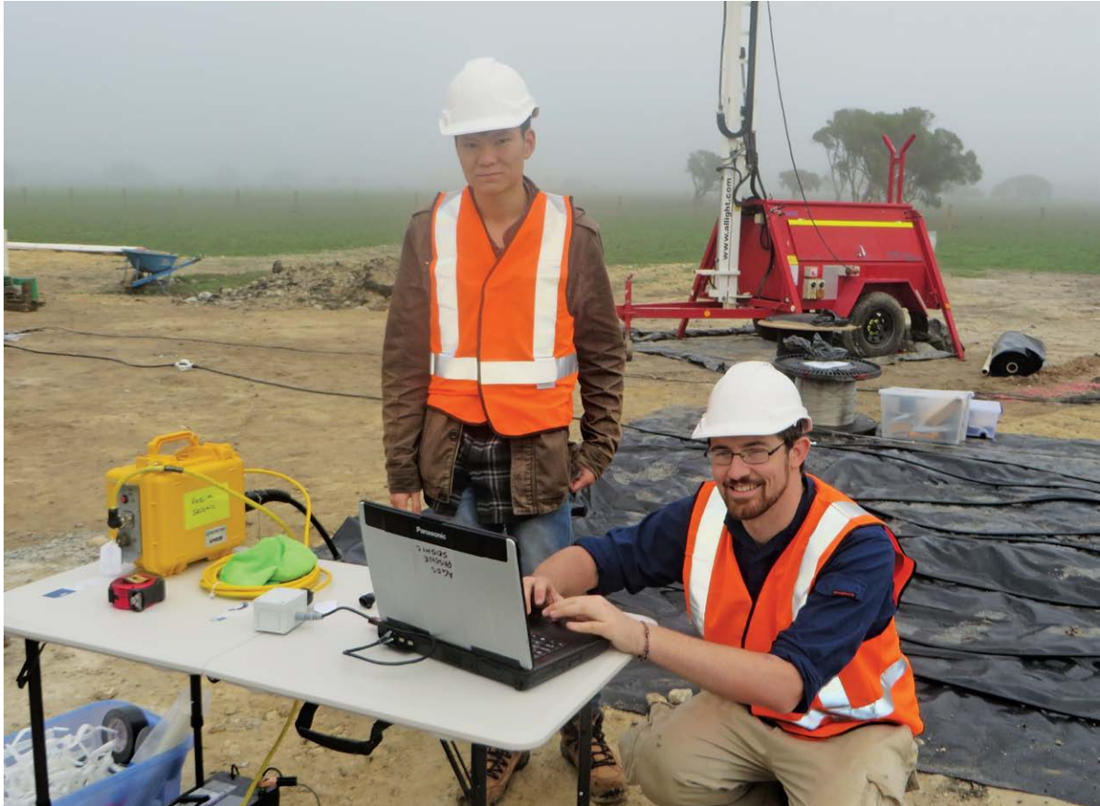
Figure 20: Preparing to deploy borehole geophone array in shallow well near Harvey 4 in the SW Hub project area. From 7-0212-0203.
