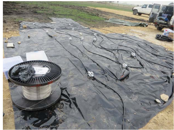
Figure 20: Preparing to deploy borehole geophone array in shallow well near Harvey 4 in the SW Hub project area. From 7-0212-0203.
