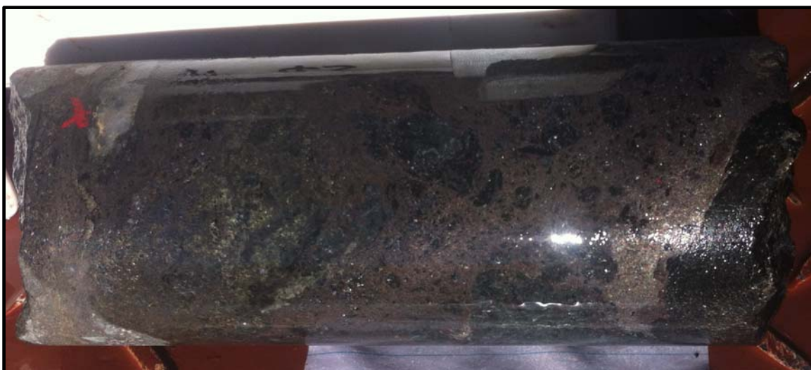
Figure 4: Sulphide (pyrrhotite) breccia 10 cm thick with minor copper (chalcopryrite) mineralisation hosted by altered mafic unit in 12AMD0018 (depth 260.15 metres) marks the base of the main mineralised zone.
