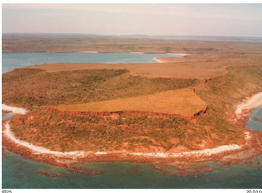
Figure 6. Photograph of bauxite deposits at Cape Bougainville, looking southward, taken from the air in 1981 during a reassessment of the deposits. The Cainozoic bauxitic duricrust profiles, forming mesa cappings, are developed over mafic volcanic rocks of the Palaeoproterozoic Carson Volcanics. Photograph courtesy Rio Tinto
