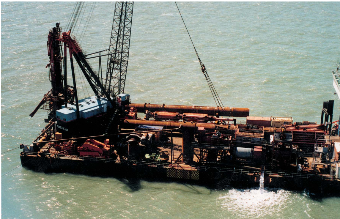
Figure 10. Photographs of offshore large-diameter drill sampling operations, northwest of Lacrosse Island: a) ship out at sea; b) large-diameter drill sampling system lies on deck of the ship. Photographs courtesy J. M. Graindorge
