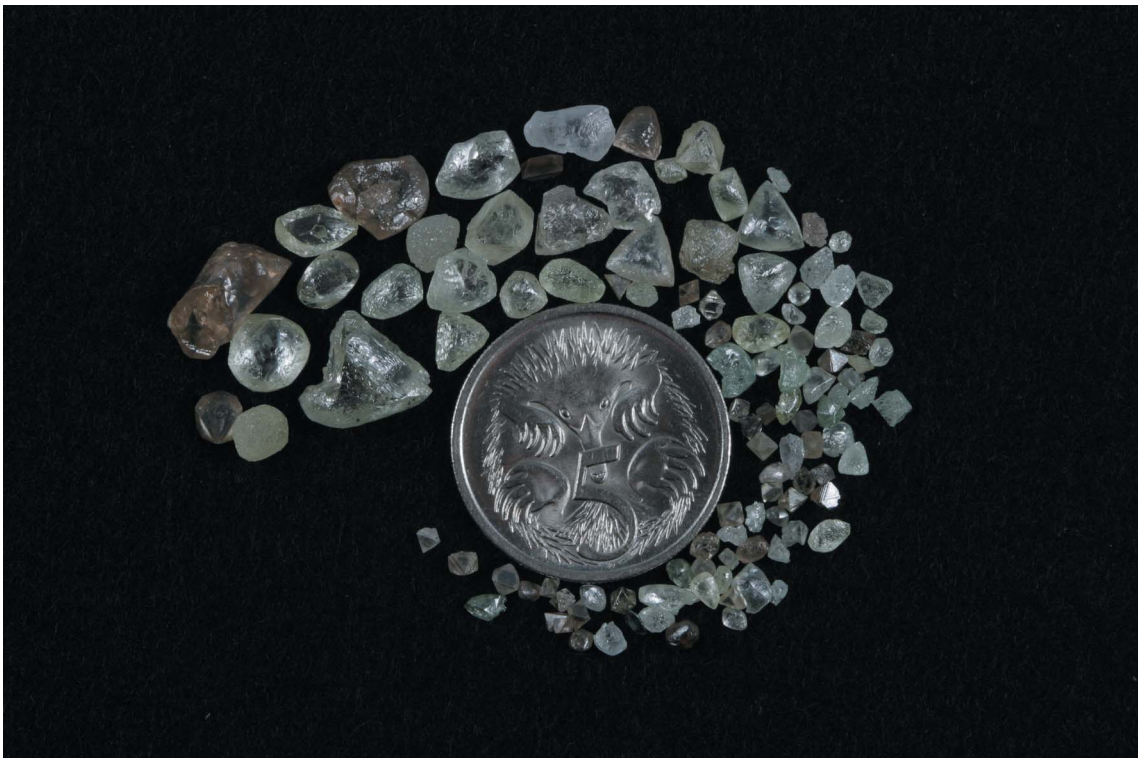
Figure 7. a) Photograph of bulk sampling pit at Southern lobe of Seppelt 1 in 2002; b) Selection of diamonds recovered from Seppelt 1 bulk sample (diameter of coin is 19 mm). Photographs courtesy Striker Resources NL
