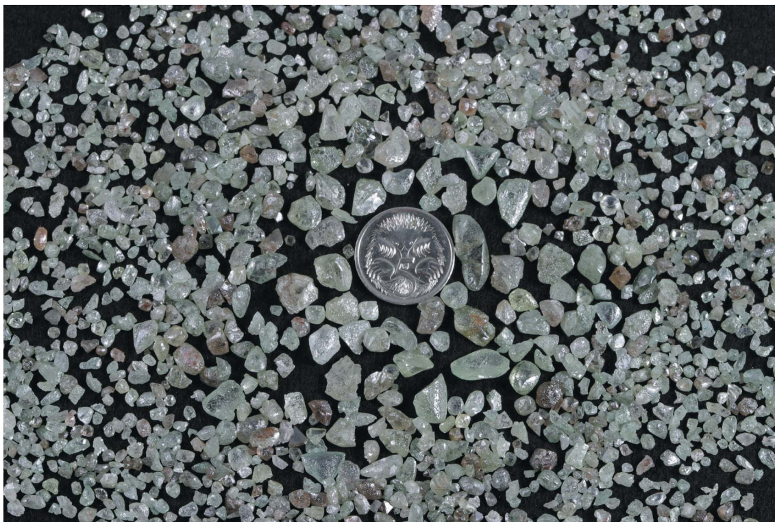
Figure 8. a) Photograph of bulk sampling pit at Seppelt 2 in 2002 (looking north); b) Selection of diamonds recovered from Seppelt 2 bulk sample (diameter of coin is 19 mm). Photographs courtesy Striker Resources NL
