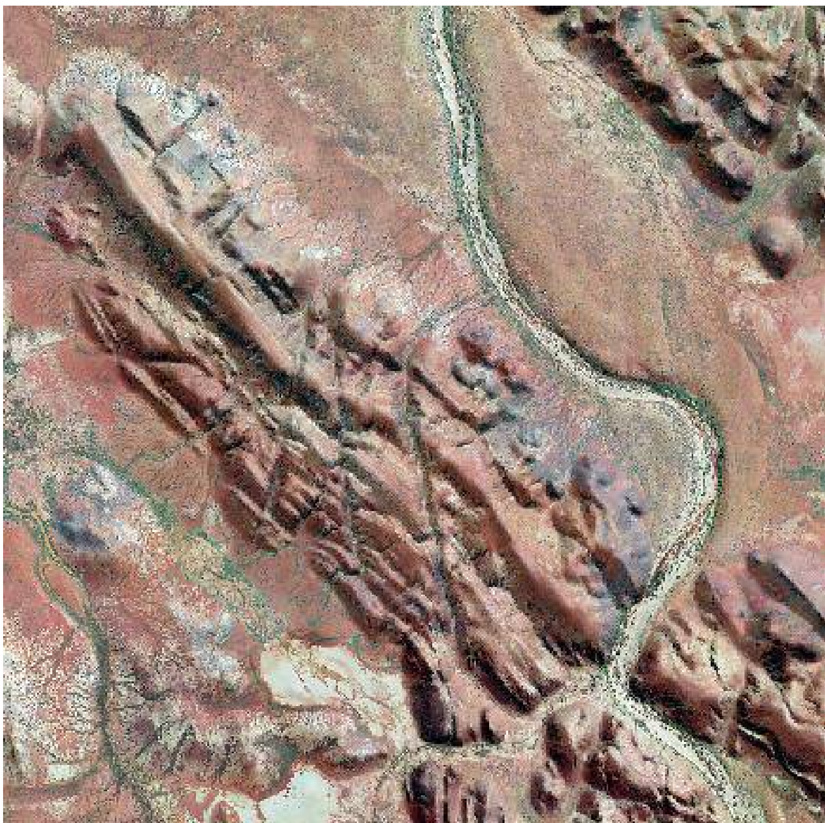
Faults offsetting resistant silicified sandstone ridges of Yilgatherra Formation and Ashburton Formation (hsortho images)
