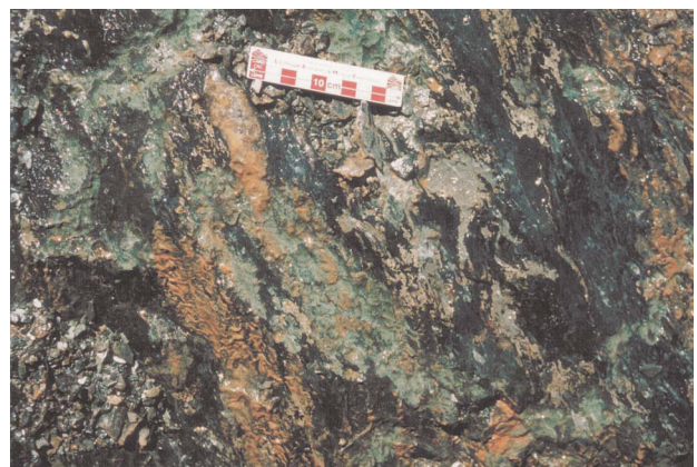
Figure 9. Detail of the chaotic internal structure of intensely sheared and chloritized Centenary Shale near the main vein
