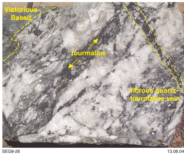
Figure 26. Slab of main vein showing extensive tourmaline replacement of laminations, and late fibrous quartz-tourmaline veins that cut the main vein fabric at a high angle
