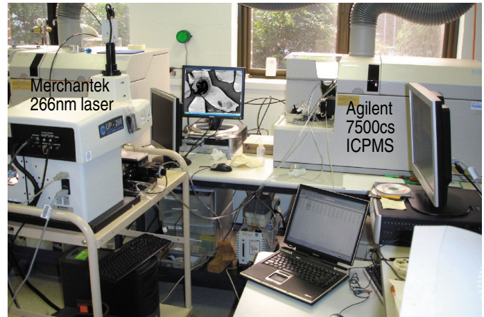
The laser ablation inductively coupled mass spectrometer (LA-ICPMS) system used at GEMOC for Lu–Hf analyses.
