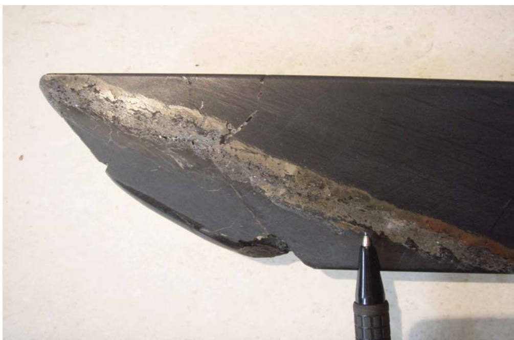
Figure 5: Sulphide-rich layer in carbonaceous pelite from EPT1174 402m.
