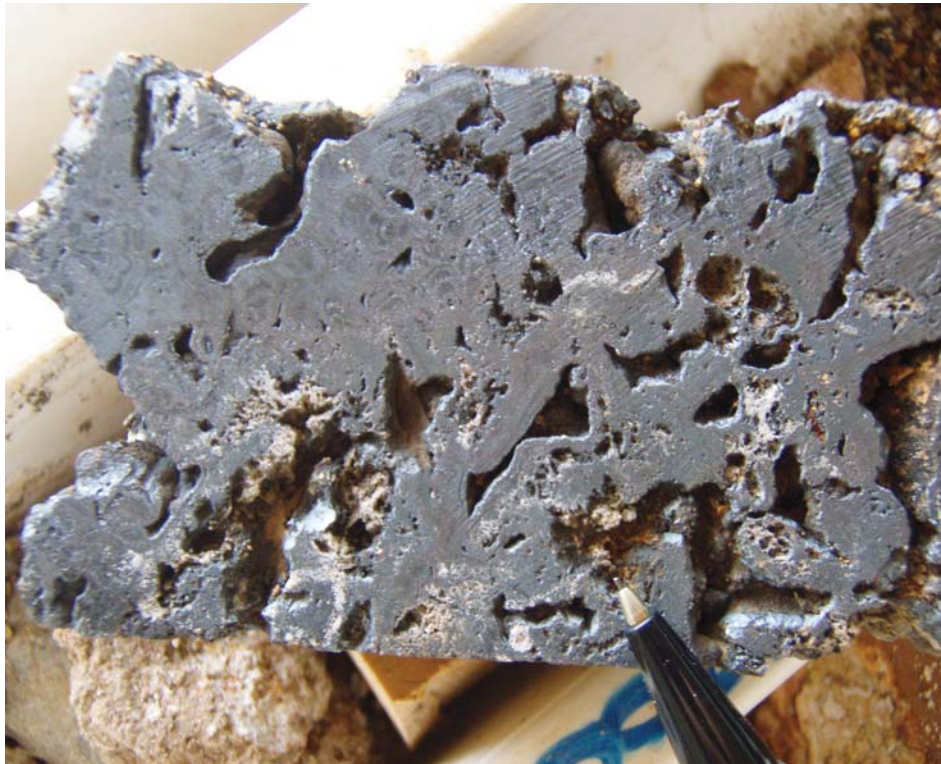
Figure 1: Void-rich colloform-textured Mn-rich material, EPT1831 200.7m. 7-8 wt.% Zn.
