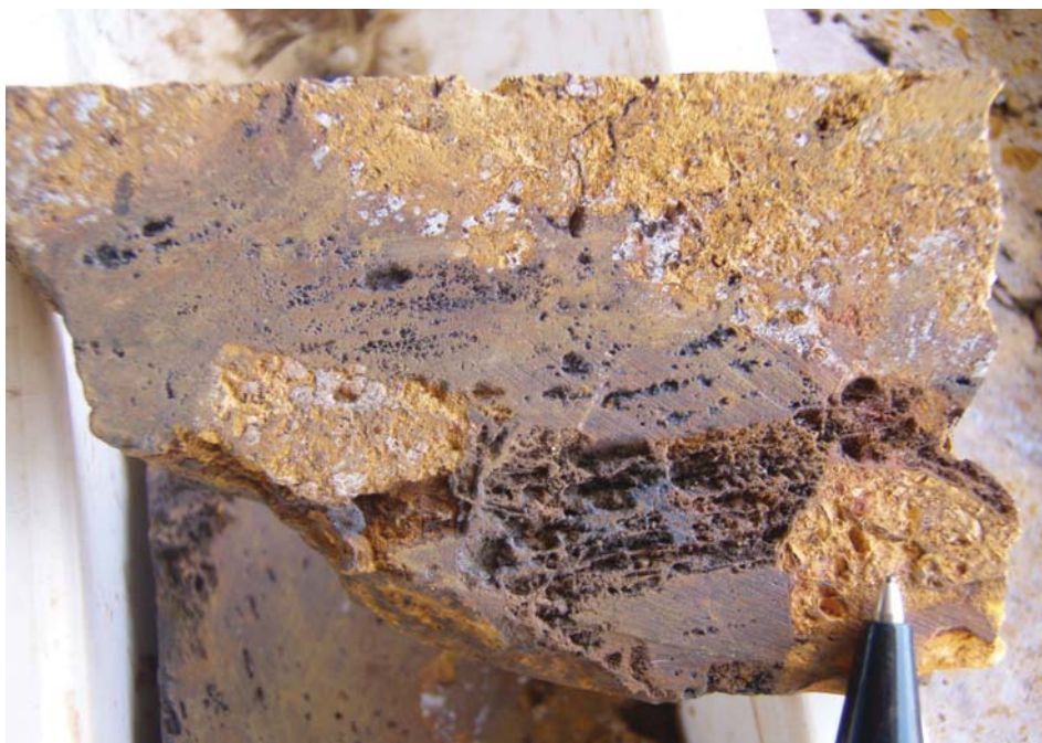
Figure 3: Brecciated gossan with boxworks, EPT1831 289.2m. Dark brown areas 1.5 wt.% Zn, light brown areas 0.6 wt.% Zn.
