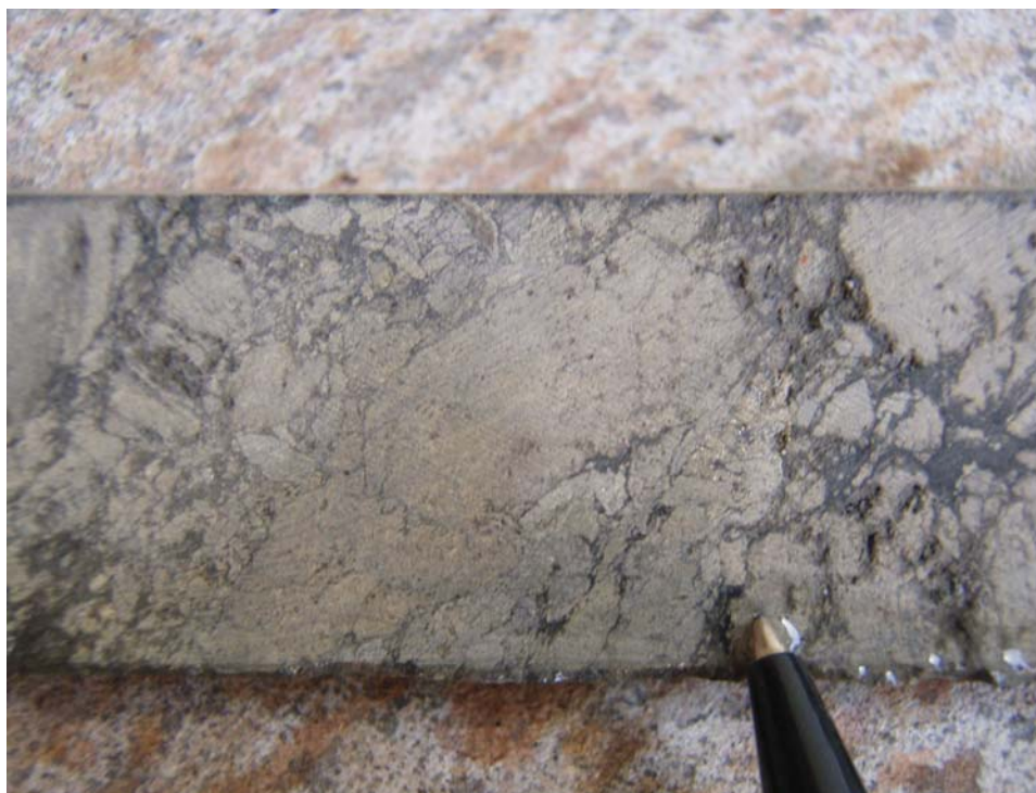
Figure 4: Massive and brecciated sphalerite from EPT1854 430.05m. 63 wt.% Zn.
