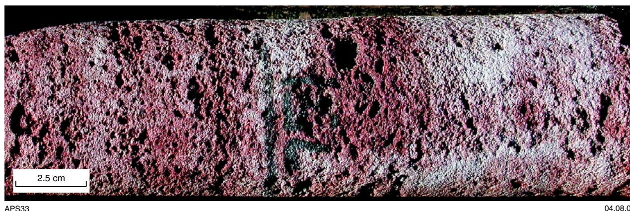
Figure 27. Photo of Hussar Formation sandstone with excellent visual porosity intersected in GSWA Lancer 1 (750–765 m)
