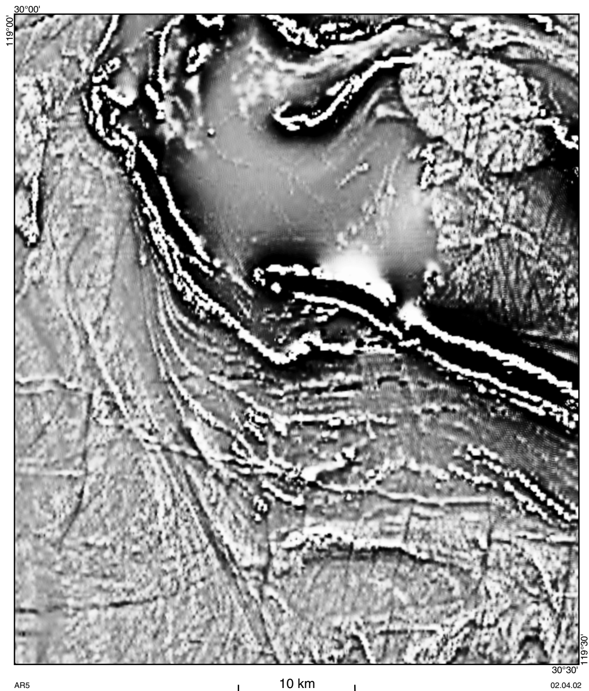
Figure 5. First vertical derivative aeromagnetic image of JACKSON (based on 400-m line-spaced data)
