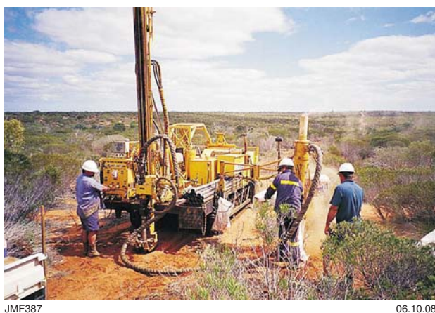
Figure 4. Air core drilling traverse over the Amy Zone of the Coburn project (after Harley, 2006)
