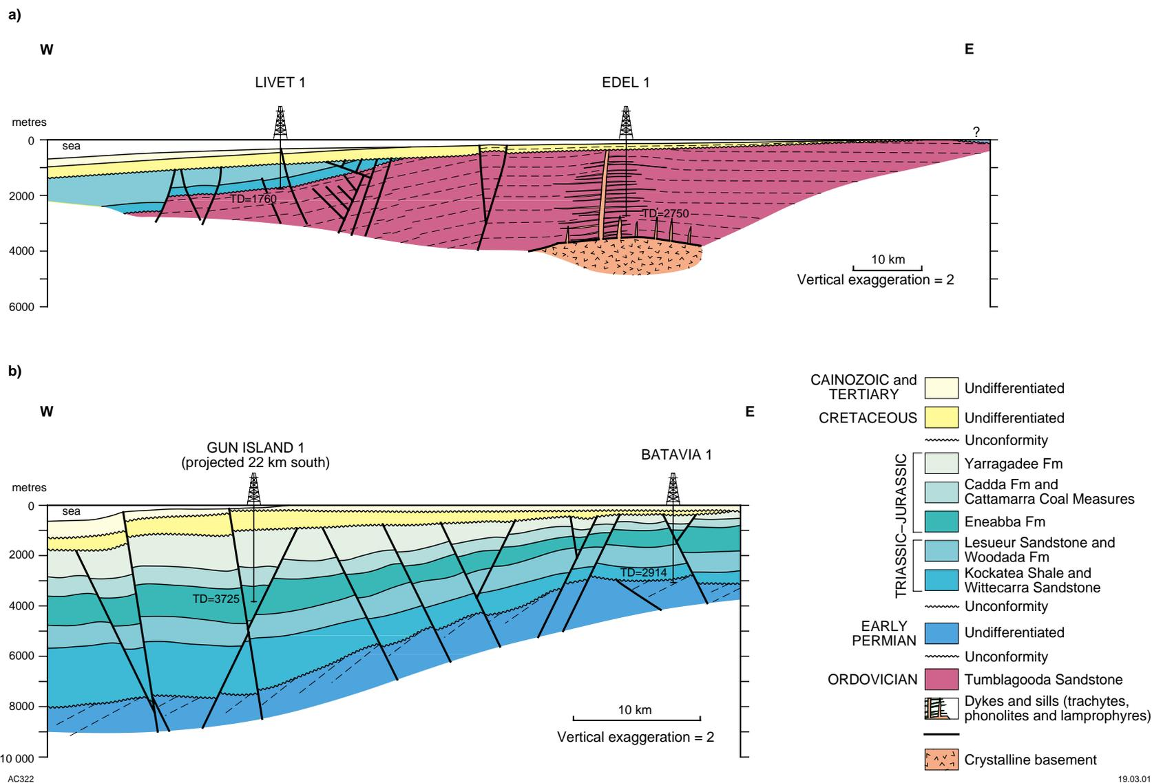
**Figure 5. Structural west-east sections across the Abrolhos Sub-basin and Edel Terrace: a) section Livet 1 to Edel 1 (from H78-110A and B seismic sections; see Figure 9), Triassic outcrop on eastern end of section projected from Kalbarri; b) section Gun Island 1 to Batavia 1 (from E92-AU09-061 seismic section; see Figure 15). Locations shown in Figures 2 and 3**
