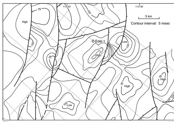
**Figure 14. Pre-drilling two-way contour map of an intra-Tumblagooda Sandstone horizon, penetrated at approximately 930 m (RT) in Edel 1 (after Ocean Ventures Pty Ltd, 1972)**
