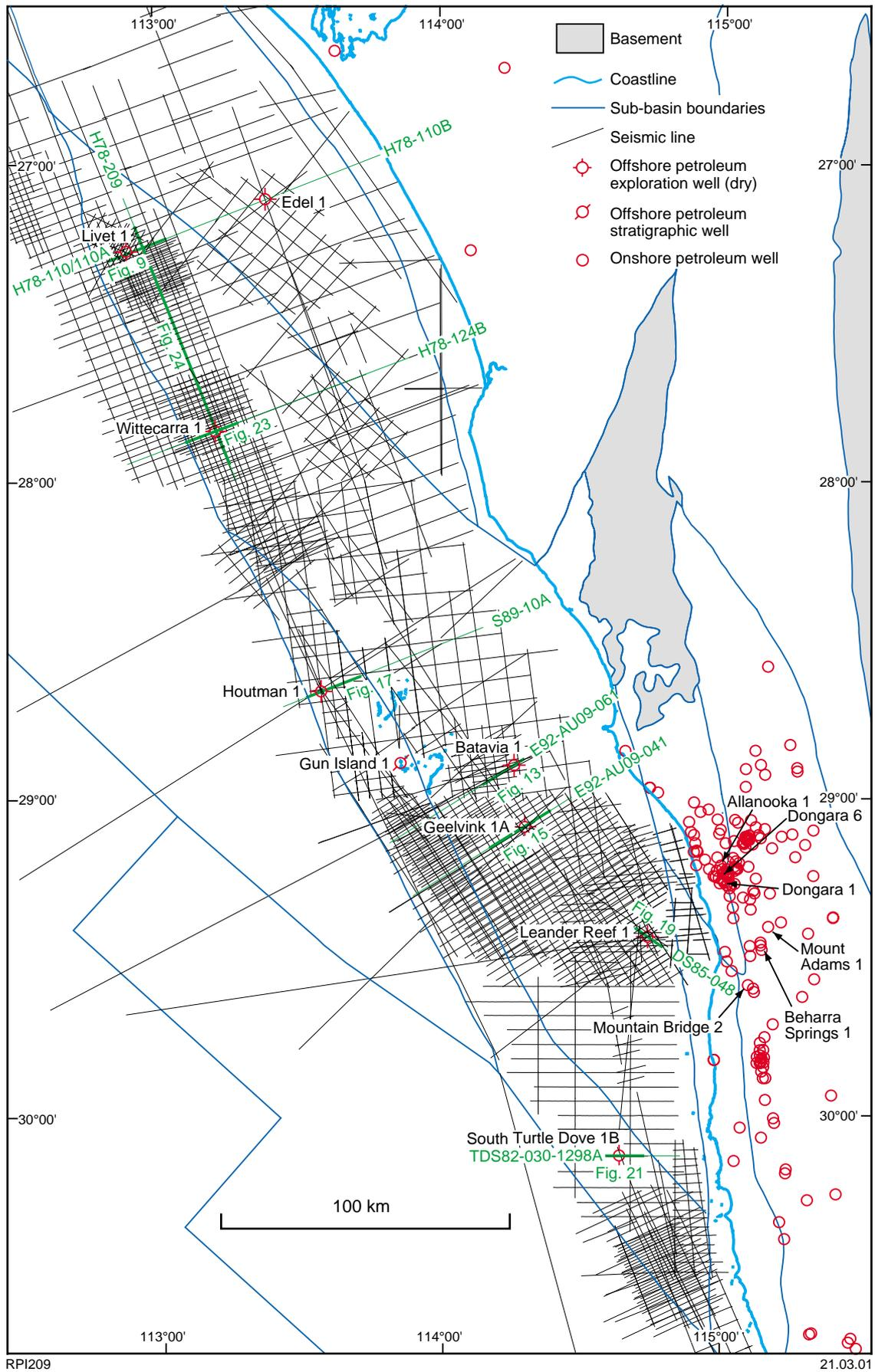
Figure 3. Seismic and well control over the Abrohlos Sub-basin. Seismic lines illustrated in this report are highlighted in green
