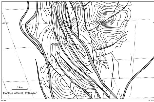
**Figure 18. Pre-drilling two-way time contour map on the top of the Permian succession for the Leander Reef area (after Diamond Shamrock Oil Company (Australia) Pty Ltd, 1984)**
