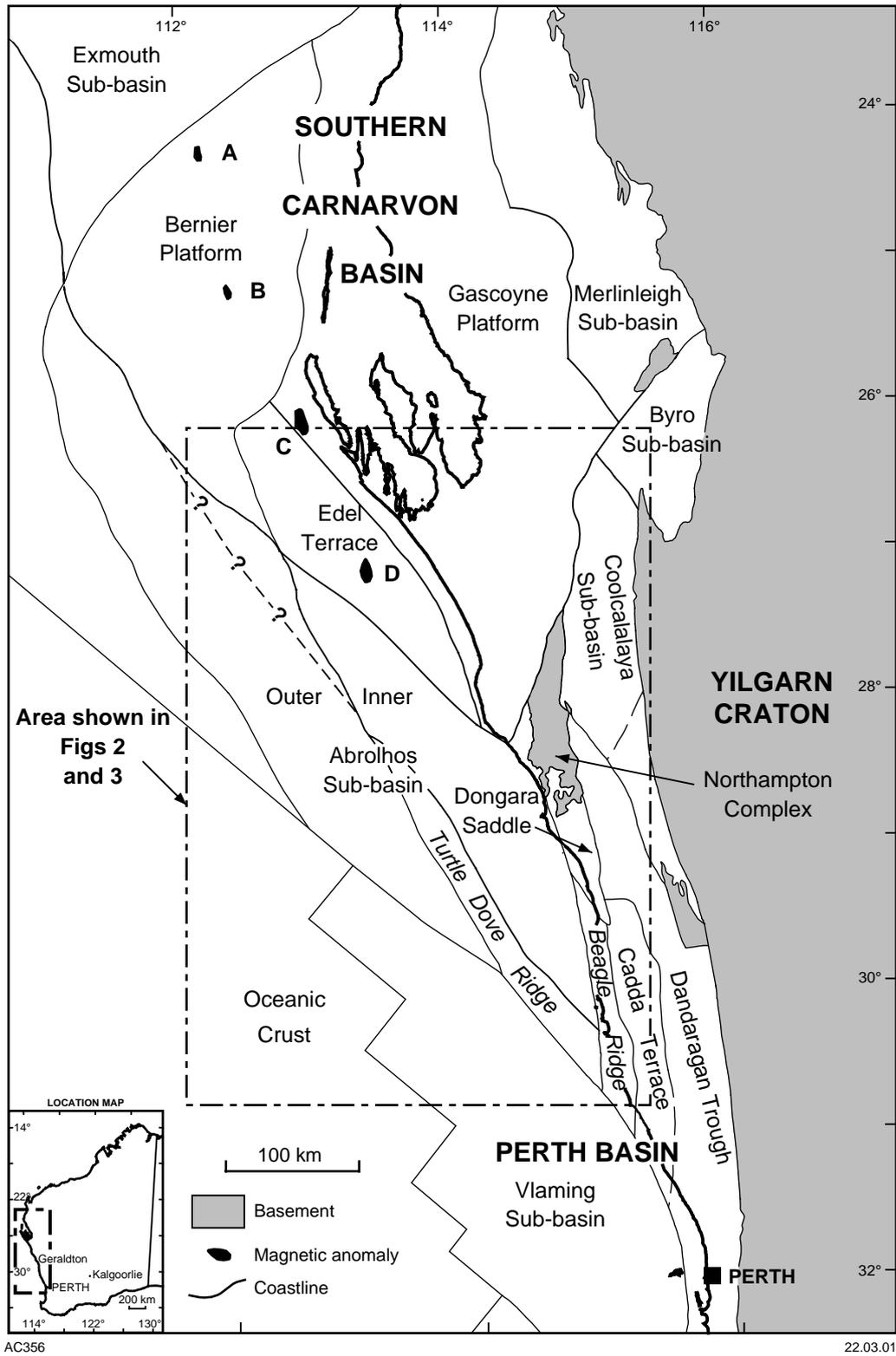
Figure 1. Regional geological setting of the Abrolhos Sub-basin. Magnetic anomalies A to D after Middleton (1993)
