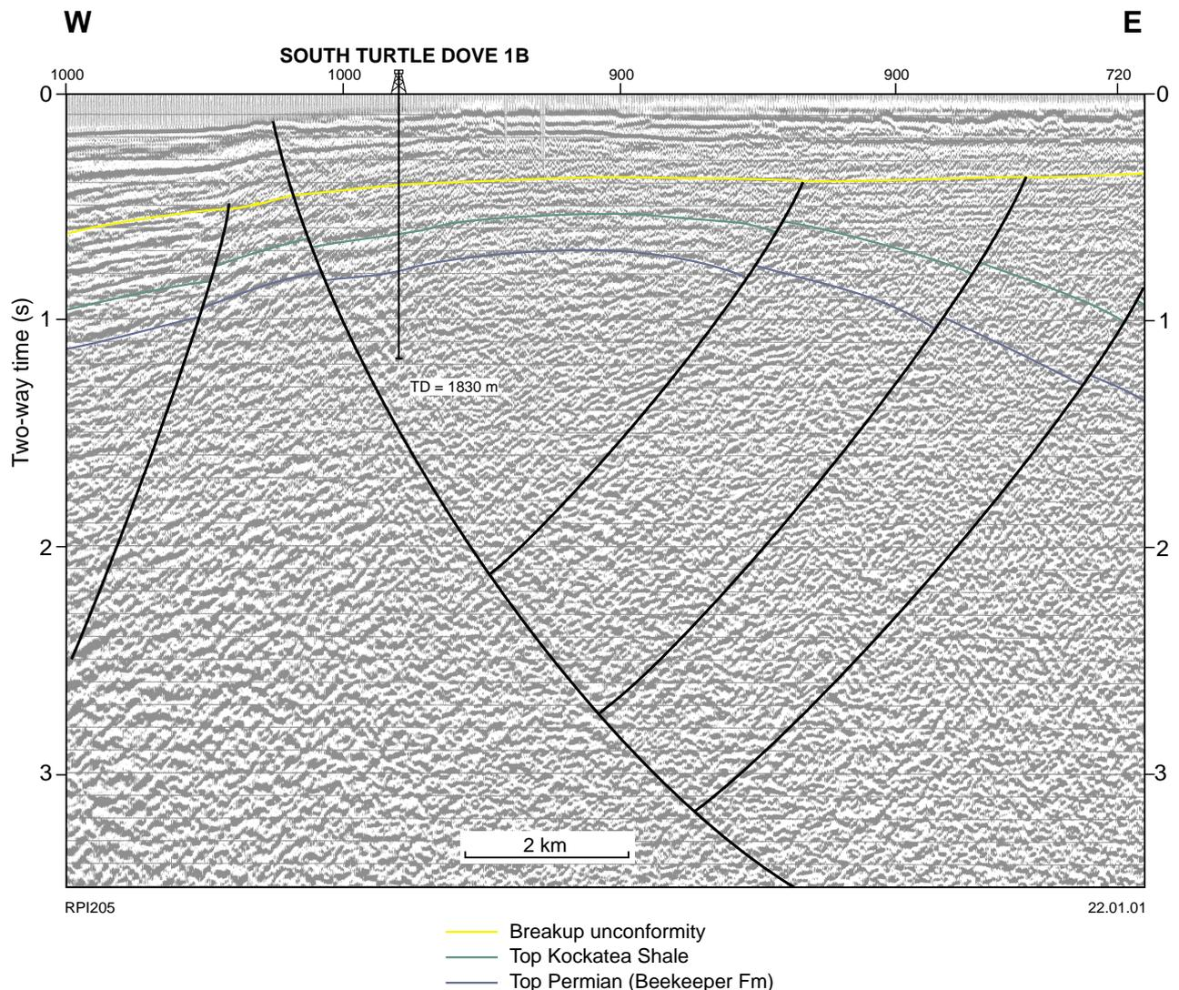
Figure 21. Seismic section TDS82-030-1298A, showing the structural setting of South Turtle Dove 1B. Location shown in Figure 3
