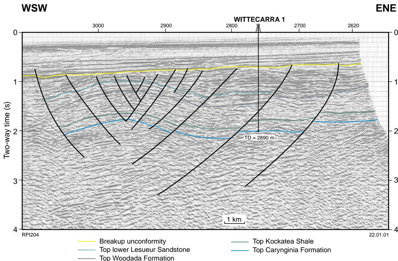
Figure 23. Seismic section H78-124B, showing the Wittecarra structure, from west-southwest to east-northeast. Location projected from 400 m west-southwest and shown in Figures 3 and 22
