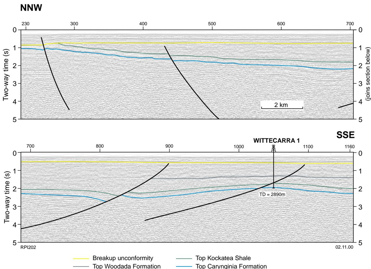
**Figure 24.** Seismic section H78-209 showing the Wittecarra structure, from north-northwest to south-southeast, with Wittecarra 1 projected east about 400 m. Location shown in Figures 3 and 22
