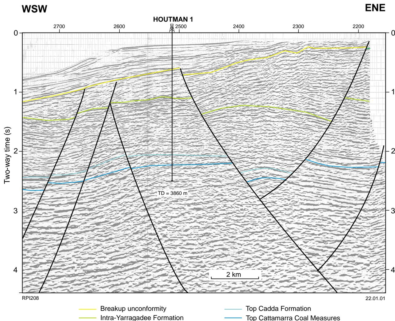
**Figure 17. Seismic section S89-10A, showing the Houtman structure. Location shown in Figures 3 and 16**
