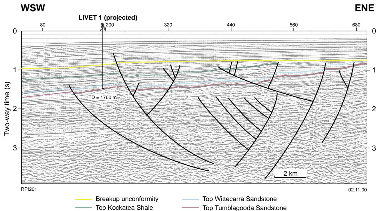
Figure 9. Seismic section H78-110A, showing the structure at Livet 1. Location shown in Figures 3 and 20
