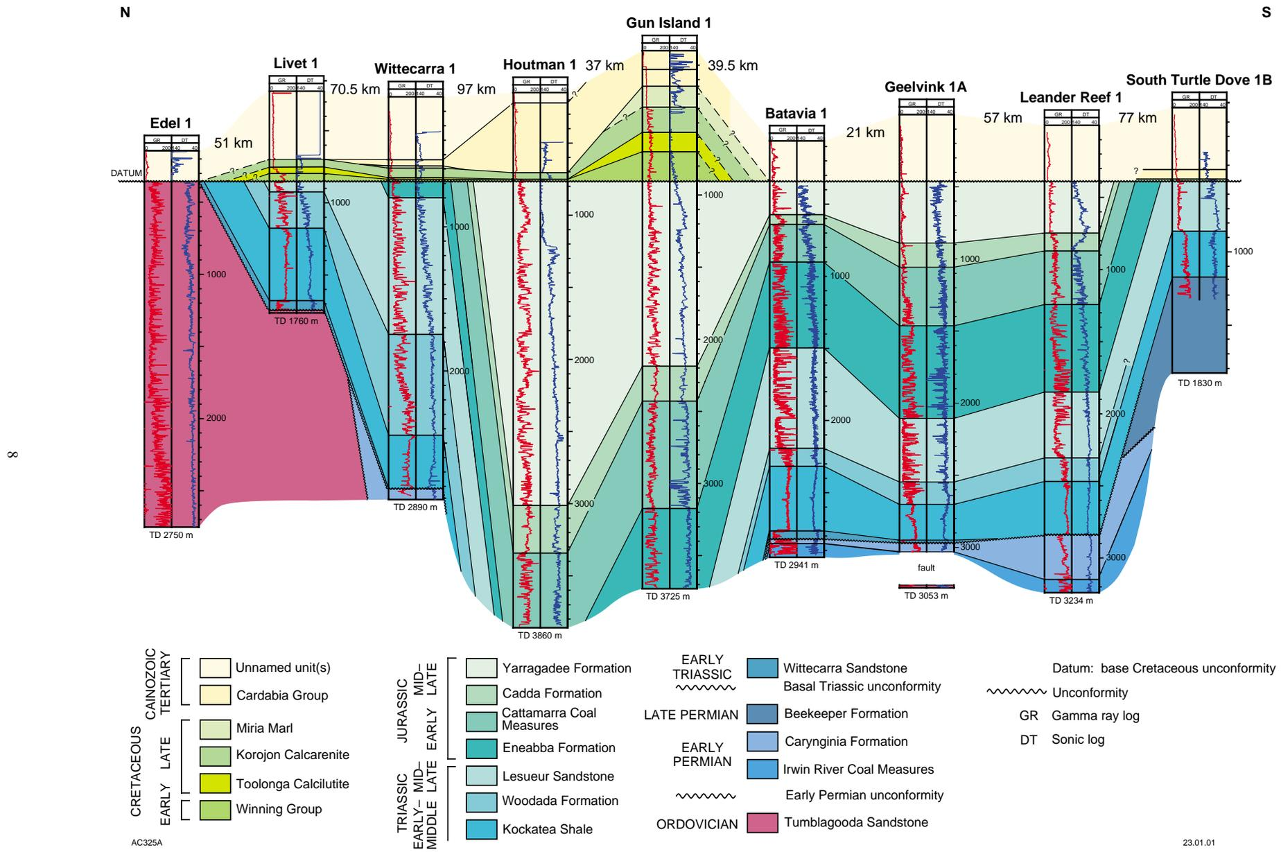
Figure 6. Simplified stratigraphic correlation along the Arohos Sub-basin. Tertiary and Cretaceous sections too poorly sampled to subdivide in some wells (after Plate 1)
