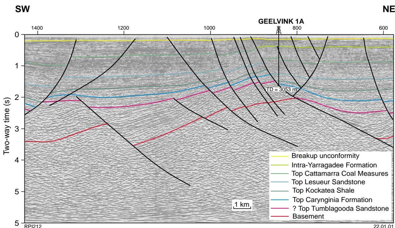
Figure 15. Seismic section E92-AU09-041, illustrating the structural setting of Geelvink 1A. Location shown in Figure 3
