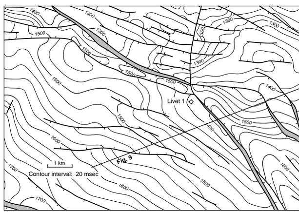
**Figure 20.** Pre-drilling two-way time contour map on the base of the Kockatea Shale in the Livet area (after Purcell and Fisher, 1997)
