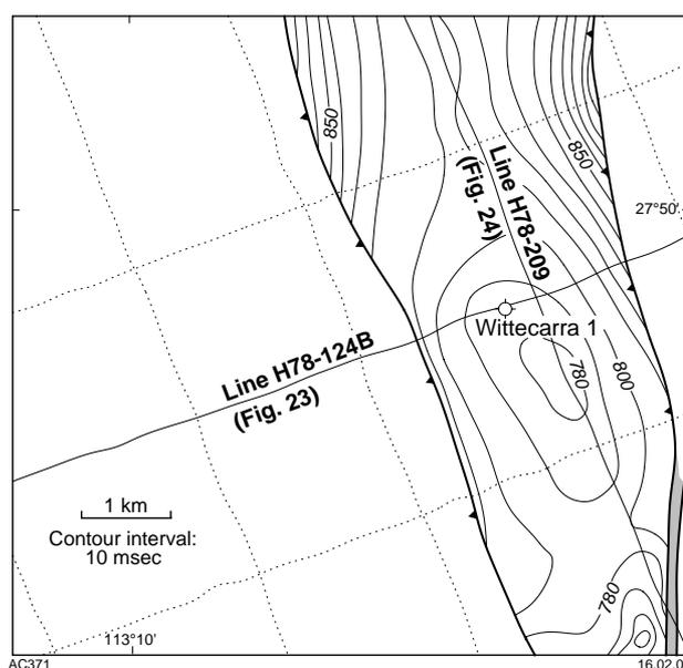
**Figure 22.** Pre-drilling two-way time contour map of the Wittecarr area on an intra-upper Lesueur Sandstone horizon (BHP Petroleum Pty Ltd, 1986)
