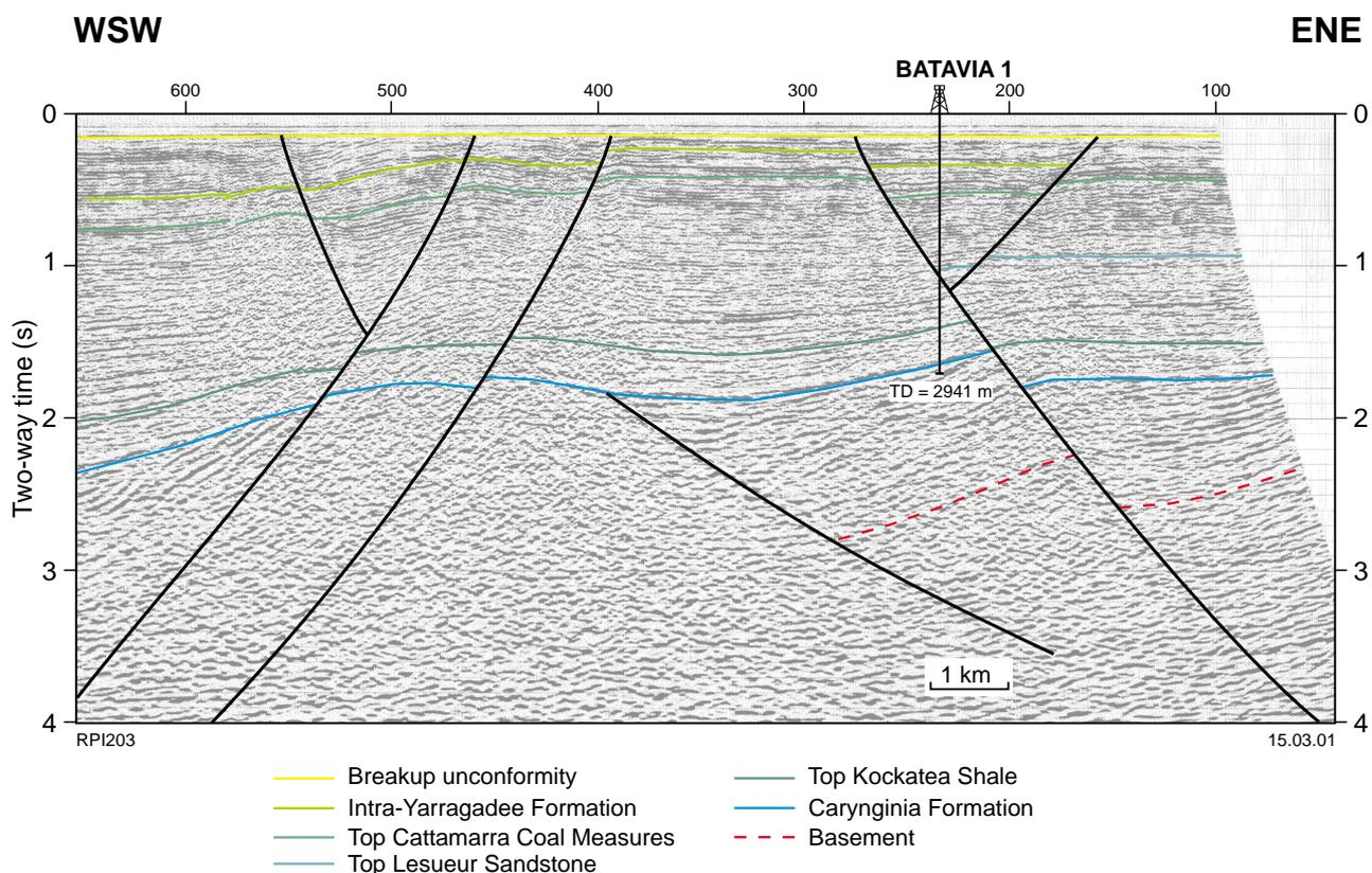
Figure 13. Seismic section E92-AU09-061, showing the structural setting of Batavia 1. Location shown in Figure 3
