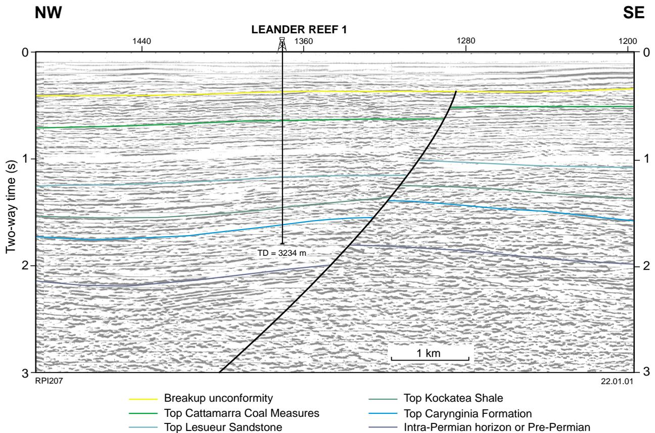
**Figure 19. Seismic section DS85-048 showing the likely structural setting of Leander Reef 1. Location shown in Figures 3 and 18**
