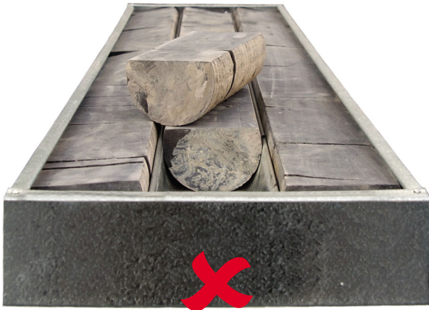
Figure 7. Heavy three-row four-inch and five-inch three-quarter core
