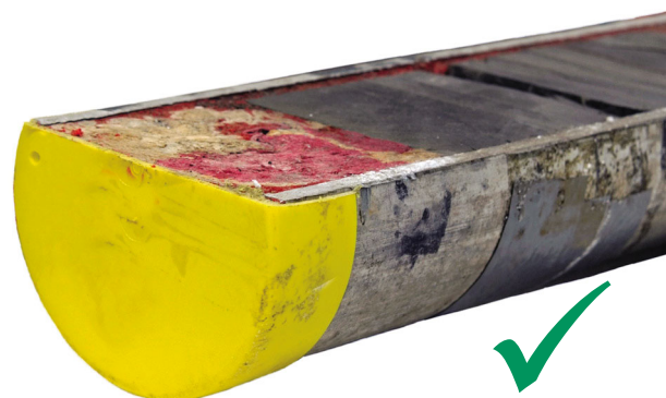
Figure 5. Tight fitting plastic end cap with cap cut to fit core barrel
