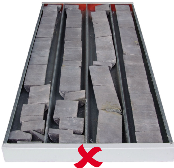
Figure 13. Undersize core for tray sections
