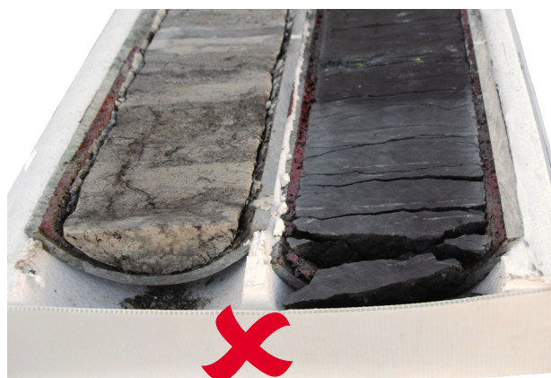
Figure 4. Core breaking away from main slab due to no end cap
