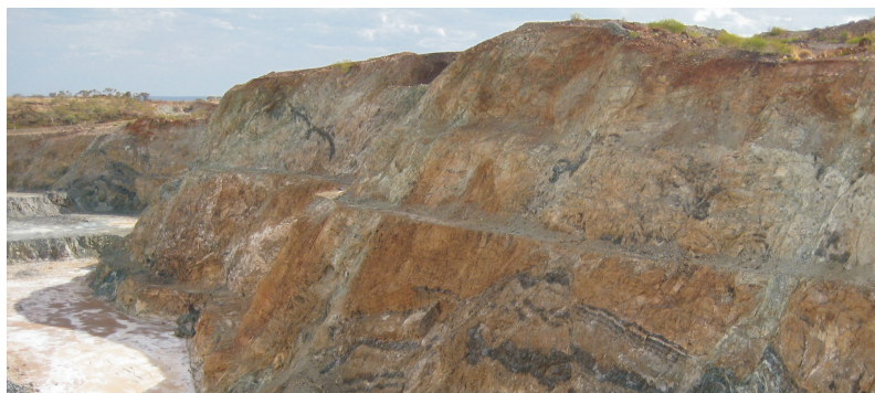
Coobina opencut mine, showing chromite lenses (Image courtesy Consolidated Minerals)
