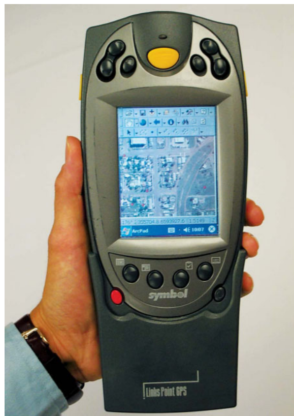
Figure 4. Symbol hand-held personal computer with the attached Links Point GPS unit
