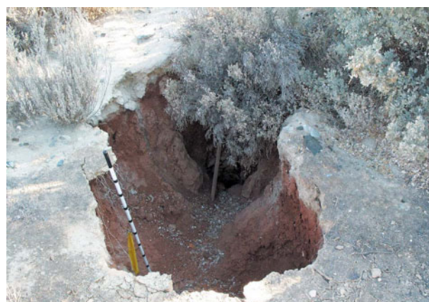
Figure 32. Large collapsed drillhole (0.5 km north of Kunanulling; Zone 51, MGA 314880E 6604500N). Stick is 1 m long
