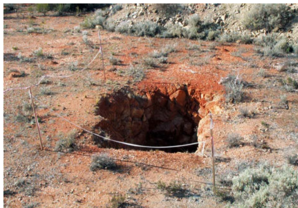
Figure 22. Shaft with no bund. The shaft is 3 m long, 1.5 m wide, and more than 10 m deep (1.5 km southeast of Broad Arrow; Zone 51, MGA 348497E 6624626N)
