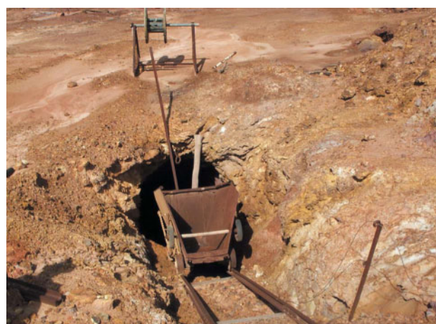
Figure 20. Inclined shaft with a 30° dip (3 km northeast of Kundip; Zone 51, MGA 240394E 6270597N)
