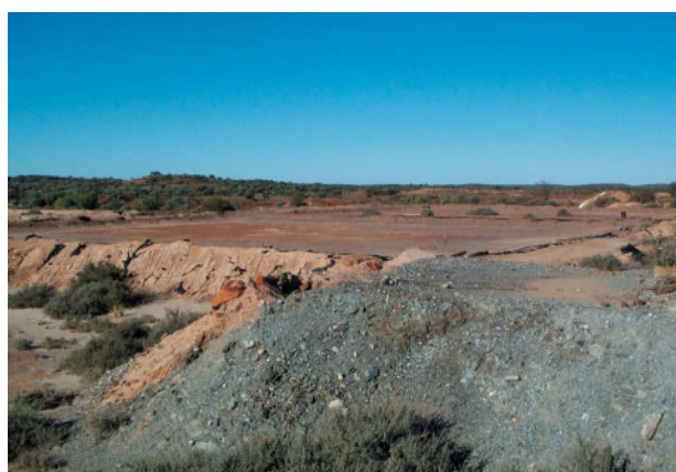
Figure 56. Typical leach pad, 75 m long, 40 m wide, and 2 m high; note the plastic lining (1.5 km south of Sandstone; Zone 50, 725744E 6900721N)
