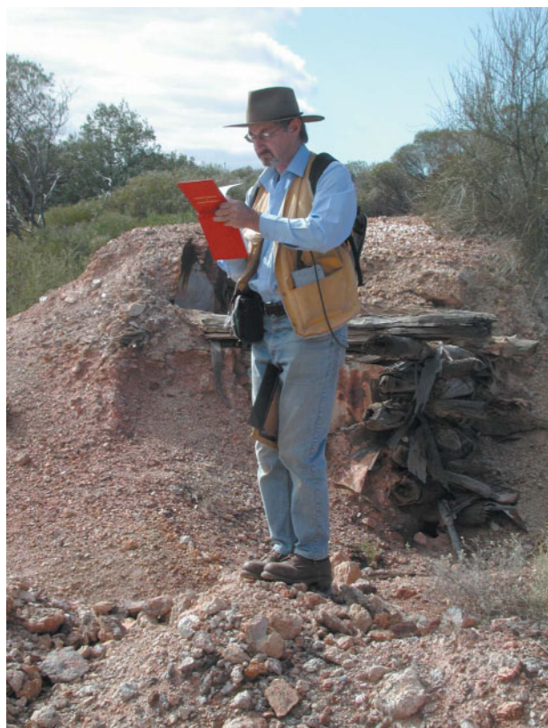
Figure 3. Geologist using a Cassiopeia hand-held personal computer in left pocket connected by cable to the Omnistar Differential Global Positioning System (DGPS) unit in the backpack
