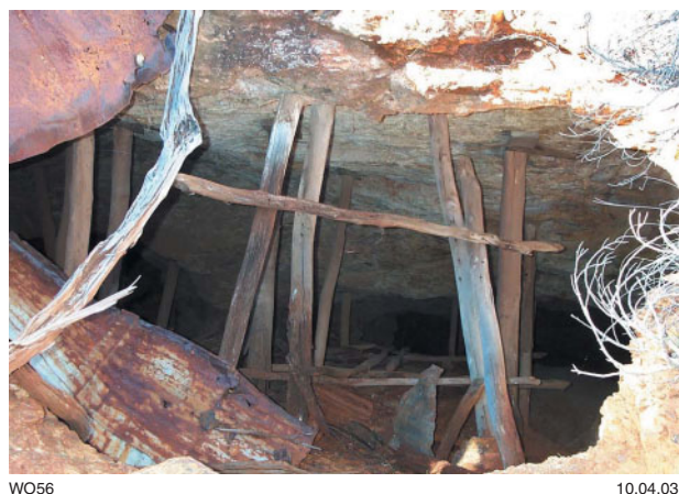
Figure 25. Open stope, 3 m long, 3 m wide, and 5–10 m deep, with a 40^\circ dip (7 km north of Coolgardie; Zone 51, MGA 323408E 6580870N)
