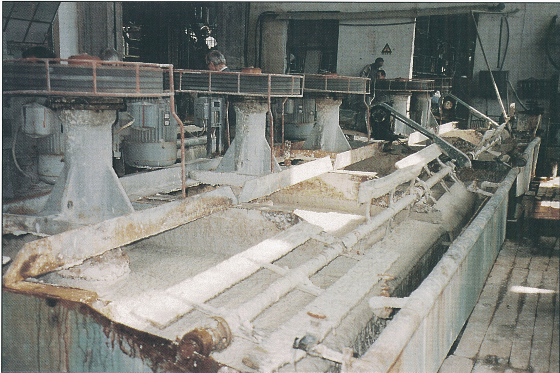
Figure 20. Fluorspar flotation circuits, Dong Feng Fluorspar Company, Zhejiang Province, China
