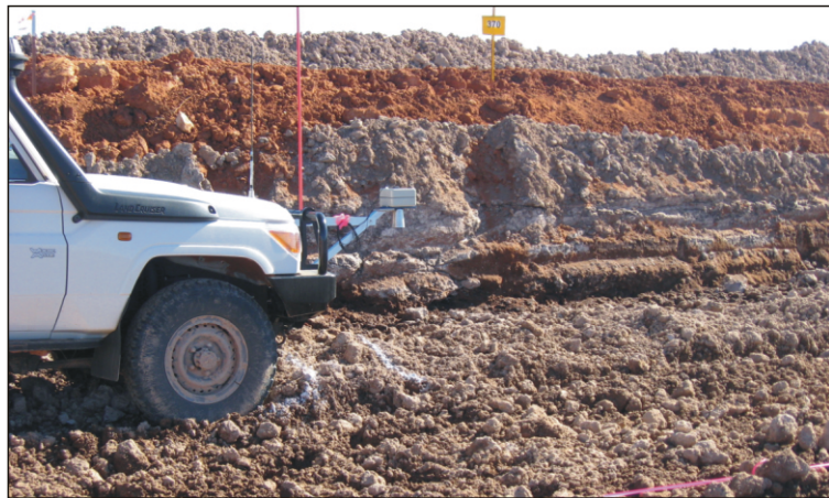
Grade control vehicle taking grade measurements, Centipede trial pit – Lake Way
