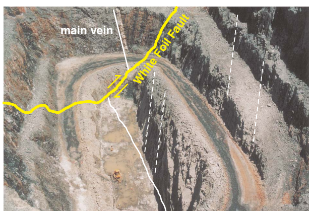
Figure 20. Location of the White Foil Fault at the southern end of the pit. Note the angular relationship between hangingwall shear zones (delineated by white dashes) in the Victorious Basalt and the main vein
