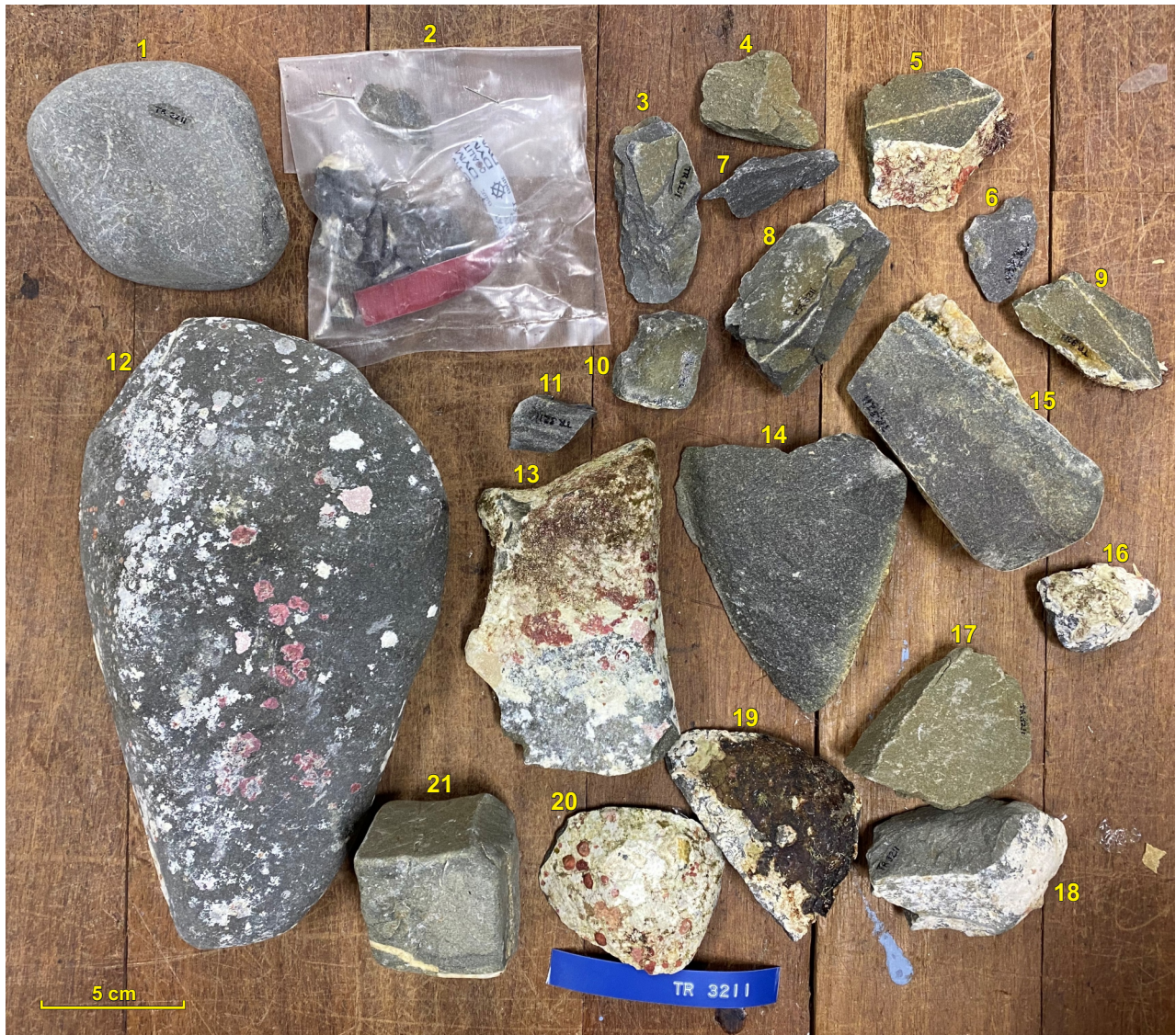
Figure 2. Ballast stones TR3211-1 to -21 recovered from the Trial Rocks shipwreck site. Specimens TR3211-5 and -9 are parts of the same ballast stone. Most stones are covered in biogenic material acquired during their residence on the sea floor
