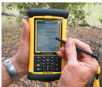
Figure 29. Field data entry using Trimble Nomad 800 GL hand-held PC
