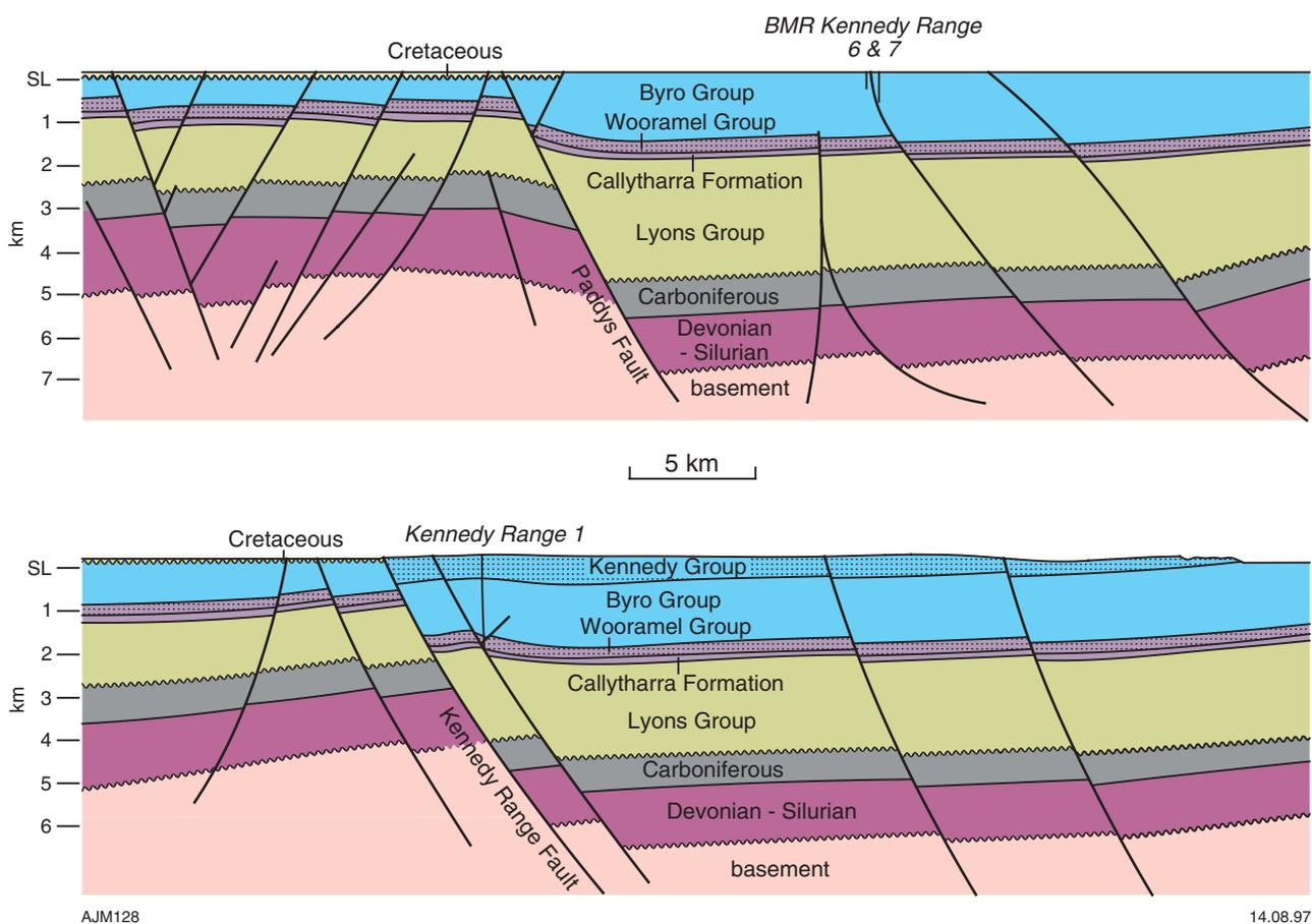
Figure 7. East-west structural cross sections through Kennedy Range 1 based on part of seismic section K82A-123, and BMR Kennedy Range 6 and 7 based on part of seismic section K82A-109.
