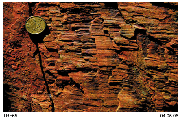
Figure 14. Quartz slickenfibres on a D_{MB3} thrust fault, Mosquito Creek Formation (MGA 250980E 7597820N). The slickenfibres at this location show a relatively consistent orientation, but in other outcrops there may be up to three sets of fibres in different orientations. View from above looking down onto a shallow-dipping fault surface
