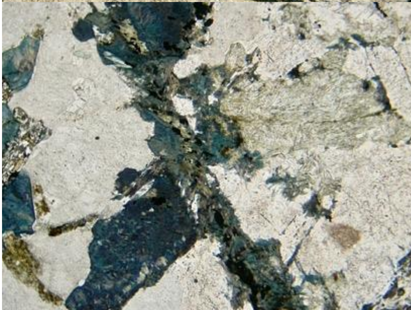
Fig. 5: Veinlike mass of blue amphibole cutting and replacing feldspar and adjacent pale green-grey amphibole aggregate (centre right). Plane polarised transmitted light, field of view 2 mm across
