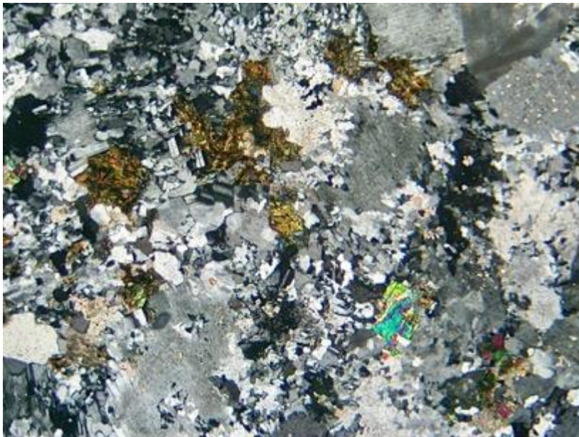
Fig. 23: Altered granitic rock, dominated by medium grained albite that is commonly finely recrystallised, plus minor aegirine (bright colours), stilpnomelane (brown) and carbonate (lower left). Transmitted light, crossed polarisers, field of view 2 mm
