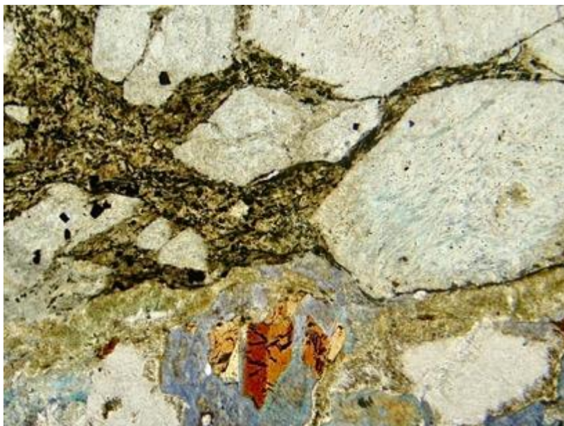
Fig. 3: Sharp contact between altered porphyritic lamprophyre (upper) and altered granitic-gneissic rock (lower). In the lamprophyre, interpreted ferromagnesian phenocrysts were replaced by very pale blue amphibole, and groundmass biotite is partly altered to chlorite. Small black grains are chromite. In the granitic-gneissic rock, there is minor residual feldspar and biotite, with replacement by blue amphibole and khaki
