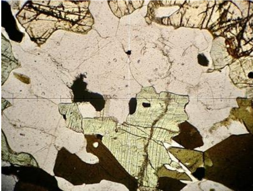
Fig. 1: Characteristic partly polygonised texture in norite-gabbro, containing plagioclase (clear), orthopyroxene (pale brown, upper), clinopyroxene (pale green), hornblende (dark brown) and magnetite (black, near centre). Plane polarised, transmitted light
