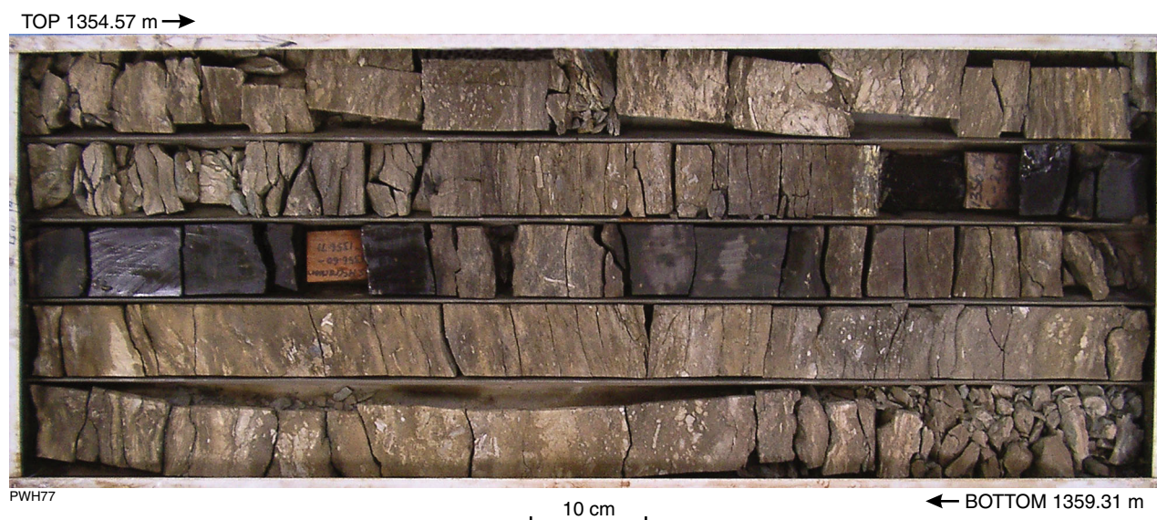
Figure 17. Drillcore photograph of Bongabinni Formation with coal-like source rock intervals (black), mineral exploration drillcore DD88SS9
