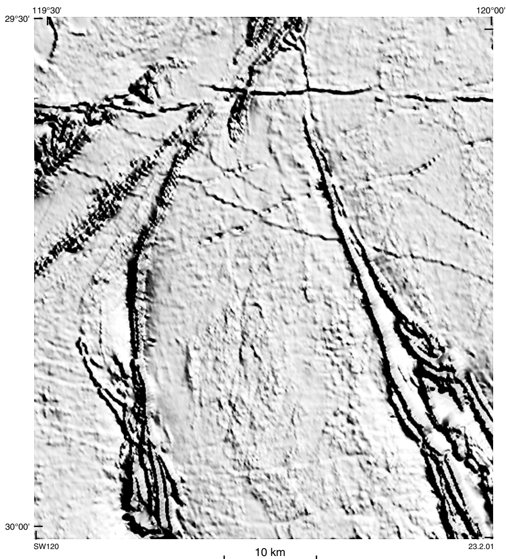
Figure 5. Total magnetic intensity image of LAKE GILES based on 400 m line-spaced data
