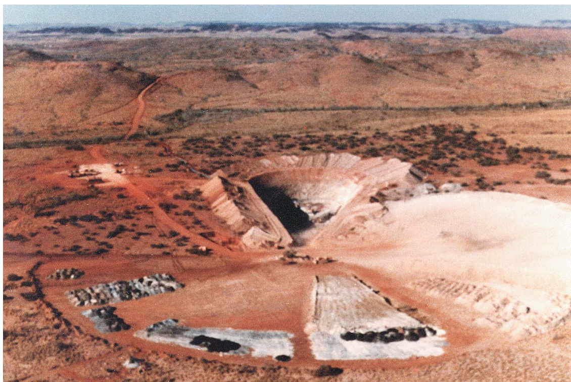
Figure 15. Photograph of Whundo openpit copper mine, looking toward the east, taken from the air in 1976 during mining of supergene ore. Photograph courtesy of Dominion Mining Ltd
