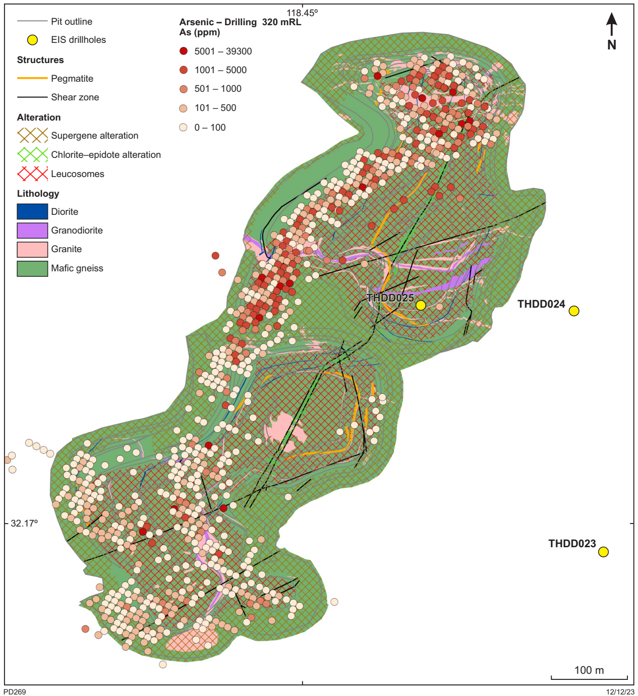
Figure. 12. Arsenic values determined for drillholes intersecting the 320 mRL horizontal surface, displayed in 1 m sample intervals
