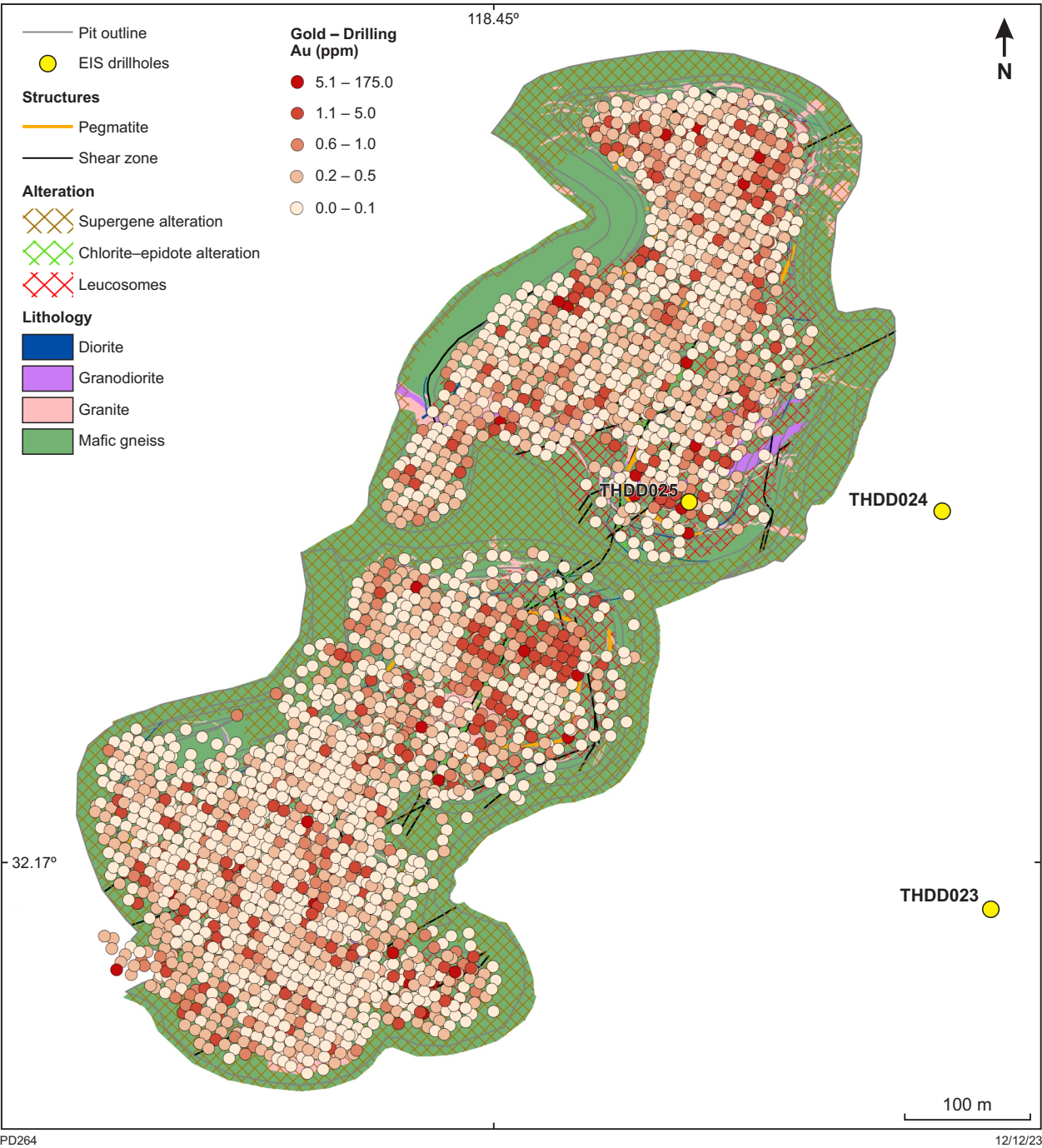
Figure 7. Gold values determined for drillholes intersecting the pit surface, displayed in 1 m sample intervals
