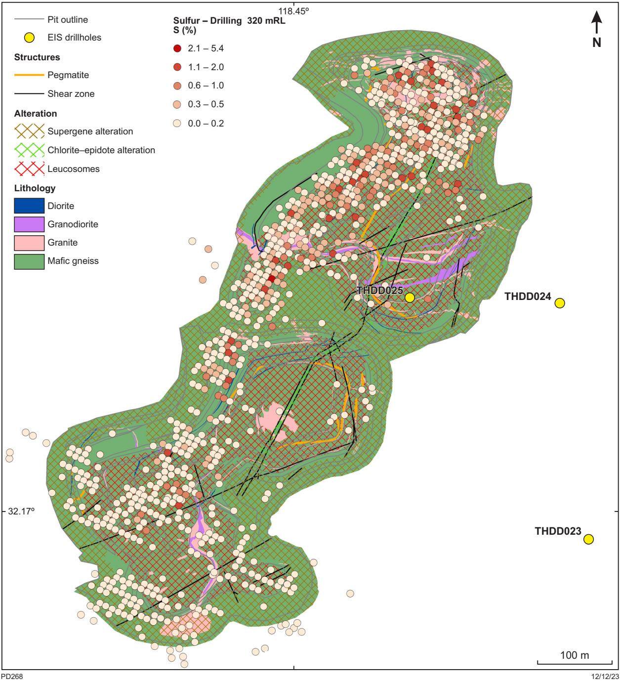
Figure 10. Sulfur values determined for drillholes intersecting the 320 mRL horizontal surface, displayed in 1 m sample intervals
