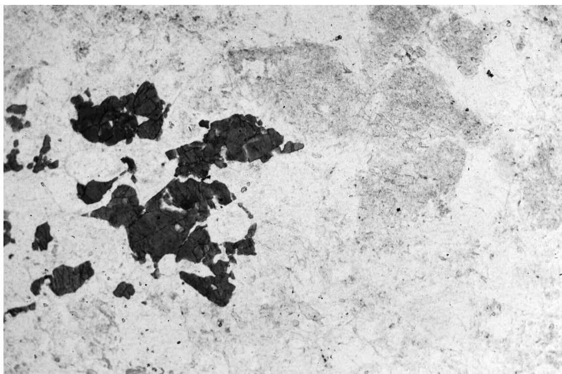
Figure 9. Photomicrograph of the Scrubber Granite taken in plane-polarized light. Field of view is 3 mm. GSWA 144728 on LANDOR (at MGA 751334). Left part of the slide shows the tourmaline–quartz(–feldspar) orbicular structure, right part of the slide shows the groundmass, which comprises quartz–feldspar(–sericite). The feldspar has a ‘dusty’ appearance, and the quartz is clear
