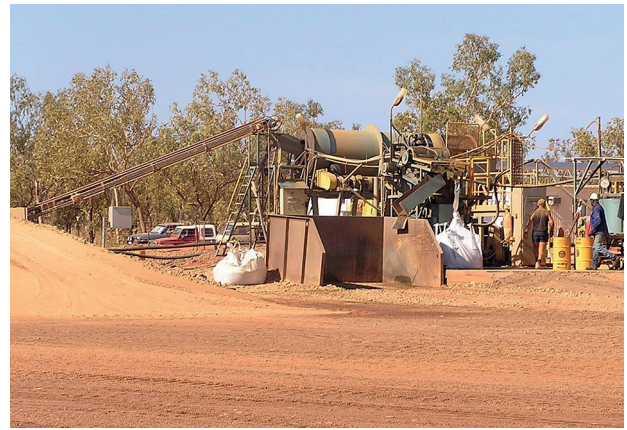
Figure 59. Blina Diamonds' 10-tph dense-media separation exploration plant (photo by D Jones)
