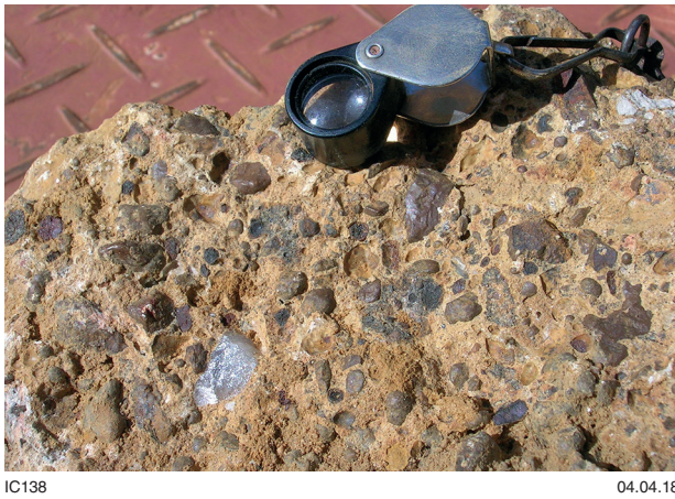
Figure 37. Basal matrix-supported gravel from BLBS201D (photo by M Hawke)
