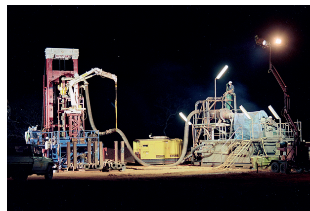
Figure 8. Large-diameter (1.4 m) drill sampling of the E4 pipe (photo by G Boxer, 1990)
