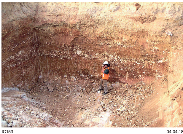
Figure 52. Northern wall of BLBS180, showing the three gravel horizons (photo by GMI Rockett)
