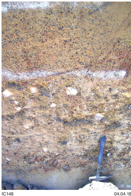
Figure 47. Pebbly clay-rich matrix-supported gravel from the central subchannel (photo by GMI Rockett)
