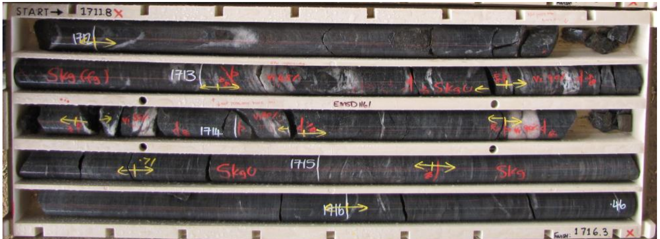
Figure 2: Core photo of the Edmunds Sandstone Contact with visible gold in quartz veins
