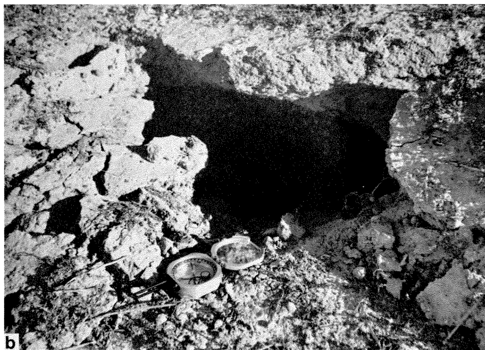
Figure 13. The Robb Fault northeast of the Shankland house: (a) note apparent left-lateral displacement of old wheel tracks and tension cracks to the rear of the collapsed scarp, (b) an exposure of the thrust plane dipping at 34^{\circ} towards 212^{\circ} (GSWA 18743)
