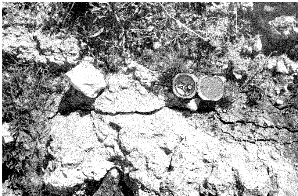
Figure 10. Tension crack in a granitic outcrop, 3 km from the southern termination of the Robb Fault (GSWA 18740)
