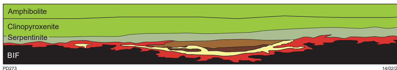
Figure 1. Massive sulfide injection into banded iron-formation (BIF) footwall and overlying metakomatiite hangingwall at the O'Toole Ni deposit, Morro do Ferro greenstone belt, Brazil (from Brenner et al., 1990)
