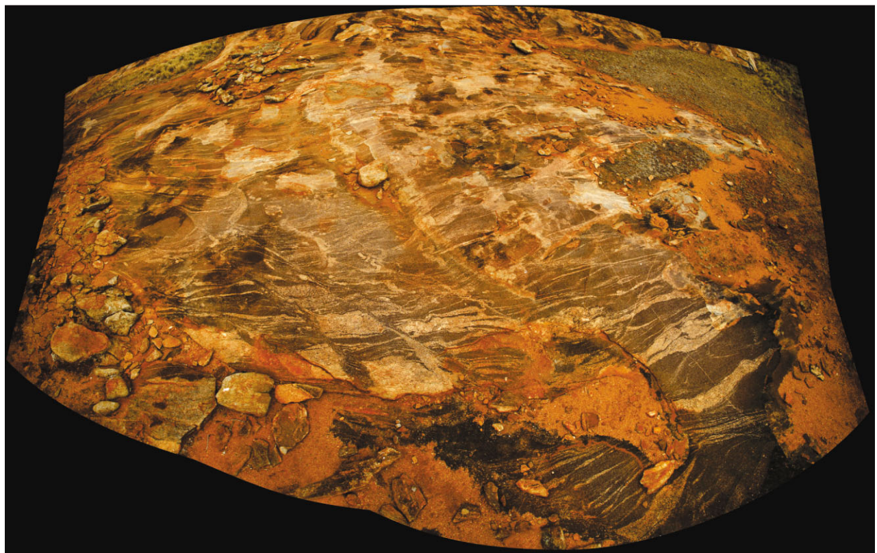
Figure 3. Megapixel image of an approximately 10 m-wide pavement of granitic bedrock in the Yilgarn Craton showing cross-cutting relationships of intrusive veins
