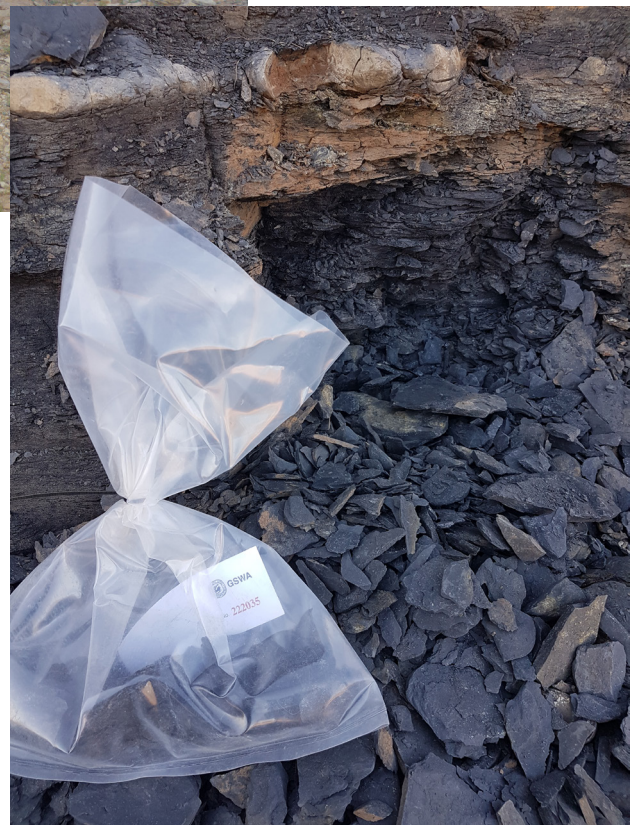
Figure 2. Rock samples collected from outcrop of the Lower Permian Bulgadoo Shale, which showed nearly 3% Total Organic Carbon. However, most of this organic matter is inertinite, making it an unsuitable source rock
