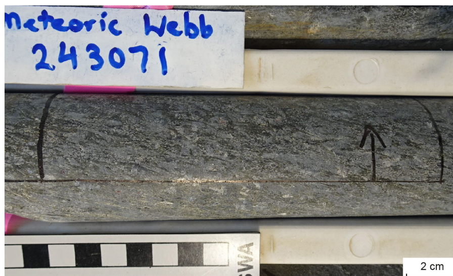
Figure 1. Drillcore image for sample 243071: garnet-bearing sillimanite–magnetite pelitic schist, Radiator prospect
