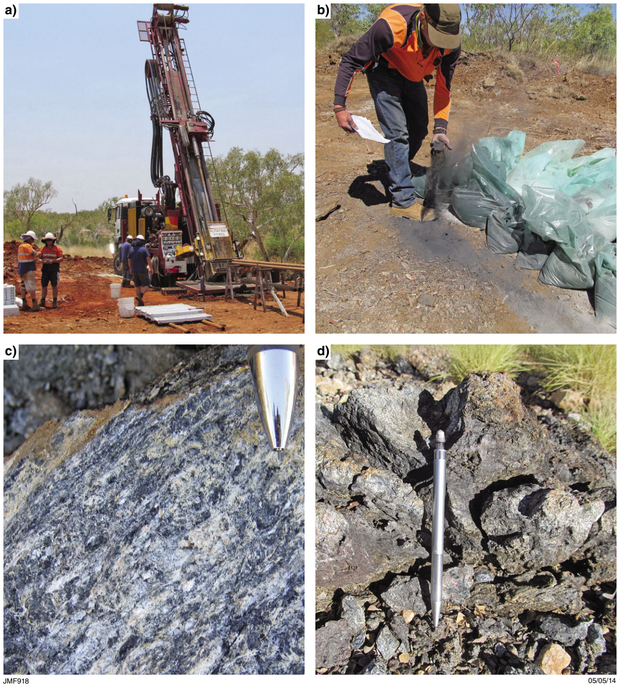
Figure 28. Exploration activities at McIntosh prospects: a) diamond drill rig in operation at Target 2; b) graphite powder sourced from a Target 1 drillhole; c) detail showing graphitic gneiss host rock at Target 2; d) surface sample of well-developed flake graphite at Target 5 (photographs courtesy Lamboo Resources)
