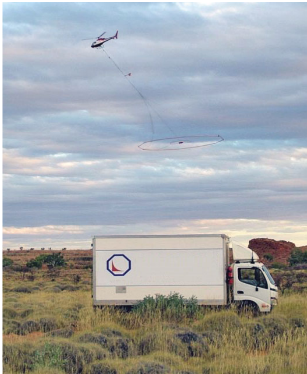
Figure 21. (left) Helicopter flying Yalbra HeliVTEM survey (Courtesy Geotech Airborne Pty Ltd, modified after Buxton Resources, 2012c)
