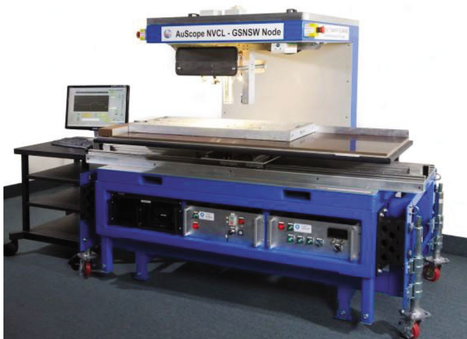
Figure 1 Picture of a HyLogger™: an integrated suite of spectroscopic, imaging, lighting, and materials handling tools (Hancock and Huntington, 2010a)
