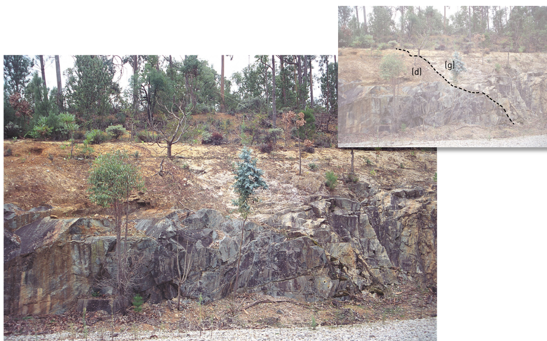
Figure 2. Contact between metagranitic rocks (g) and the main dolerite dyke (d) in the Jarrahdale railway cutting (MGA 414735E 6426400N) traceable through the lateritic profile
